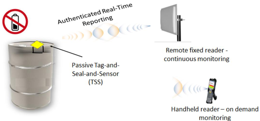
*FIG.2. Concept of operations for long-range passive (battery-free) tag-and-seal-and-sensor with data and physical security. Continuous monitoring can be performed using the remote fixed readers, and on-demand monitoring is available with handheld readers.*
