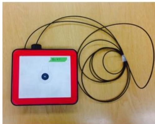
*FIG.4. Passive TSS is equipped with self-destruction upon removal capability to prevent cloning threats.*
