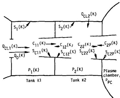
Fig. 2. Typical two-chamber tank system K showing the notation used; the general case of tapered ducts with internal cryopanel is assumed.
