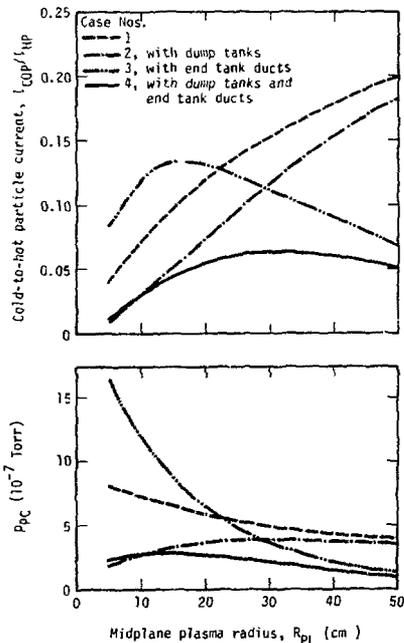
Fig. 4. Effect of configuration changes of the MX vacuum system on the ratio of cold-to-hot particle currents impinging on the plasma.
