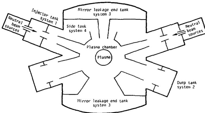
Fig. 1. Schematic diagram of the MN experimental mirror machine illustrating the multi-chamber vacuum system.
