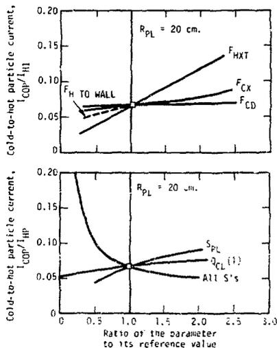
Fig. 5. Sensitivity of the ratio of cold-to-hot particle currents impinging on the plasma to variations in some of the MK vacuum system and plasma parameters.
