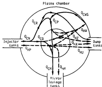
Fig. 3. Simplified flow diagram for the principal hot and cold particle flows.
