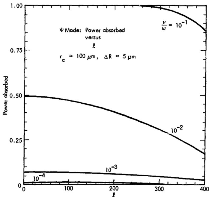
Figure III.7  $\psi$  mode: Power absorbed versus  $l$
