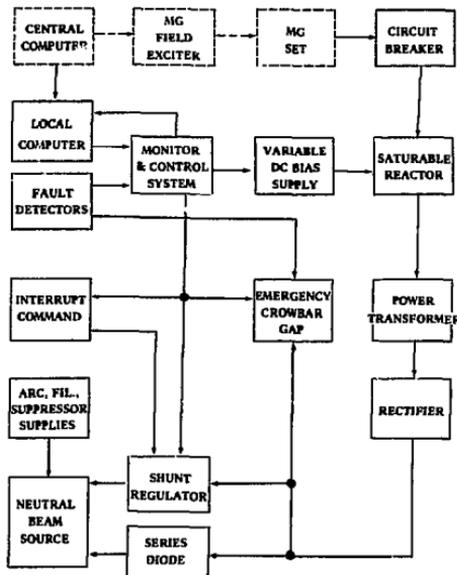
Figure 1. Block Diagram of Power Supply System for TFTR Neutral Beam Source
