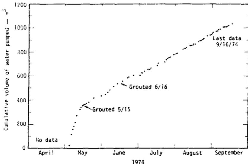
Fig. 4. Cumulative amounts of ground water pumped from hole U2aw, 1974 (Ref. 5).
