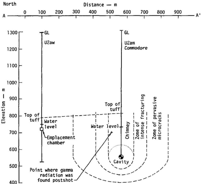
Fig. 8. Cross section showing relationships between *Commodore* (U2am) and emplacement chamber in U2aw.
