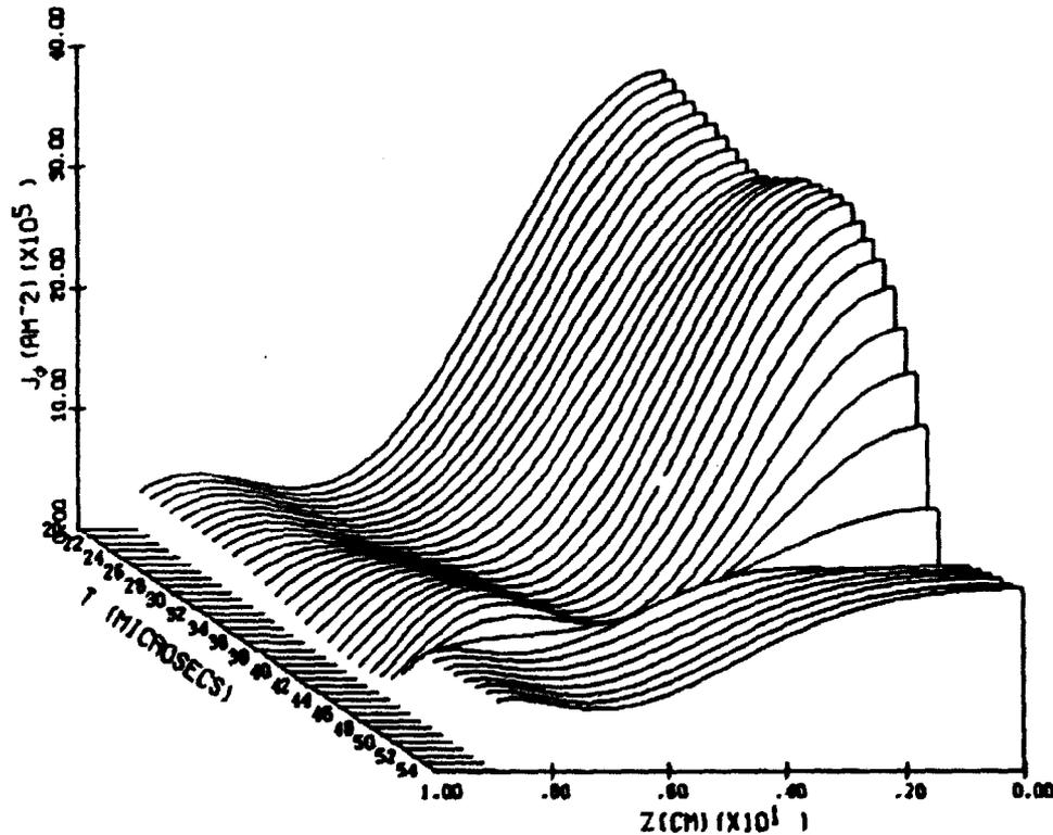
Figure 3. Evolution of toroidal current density
