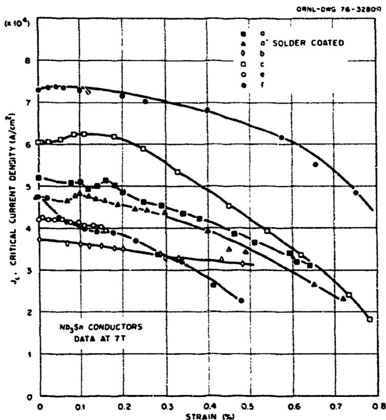
Fig. 3. Critical Current Density as a Function of Apparent Strain. (Legend letters refer to Fig. 1).
