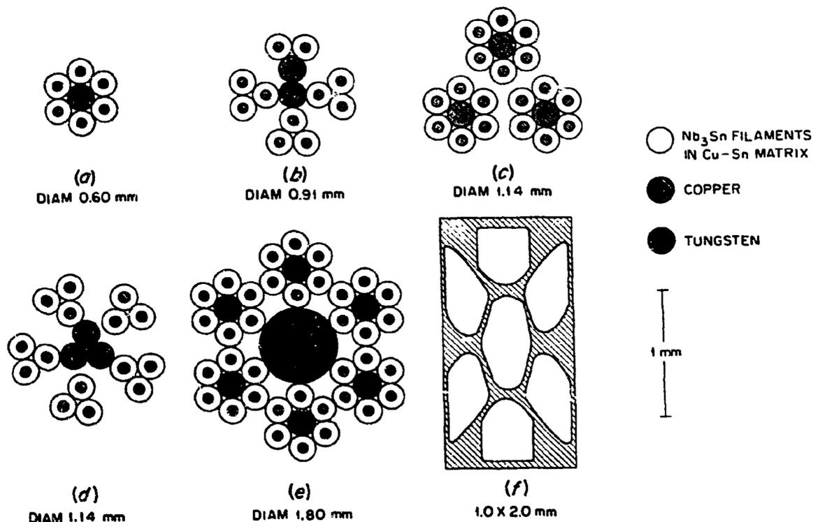
Fig. 1. Multifilamentary  $\text{Nb}_3\text{Sn}$  Conductors.
