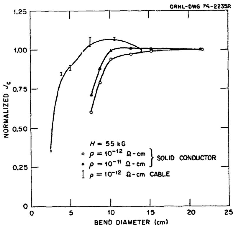
Fig. 2. Critical Current Density Normalized to Unbent Sample Value Versus Bend Diameter. (a) 1- x 2-mm monolithic sample. (b) 36 strand cable with tungsten cores.
