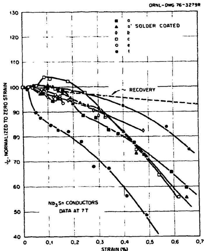
Fig. 4. Critical Current Density Normalized to Zero Strain Versus Apparent Strain. Dashed line indicates approximate values obtained upon release of load.
