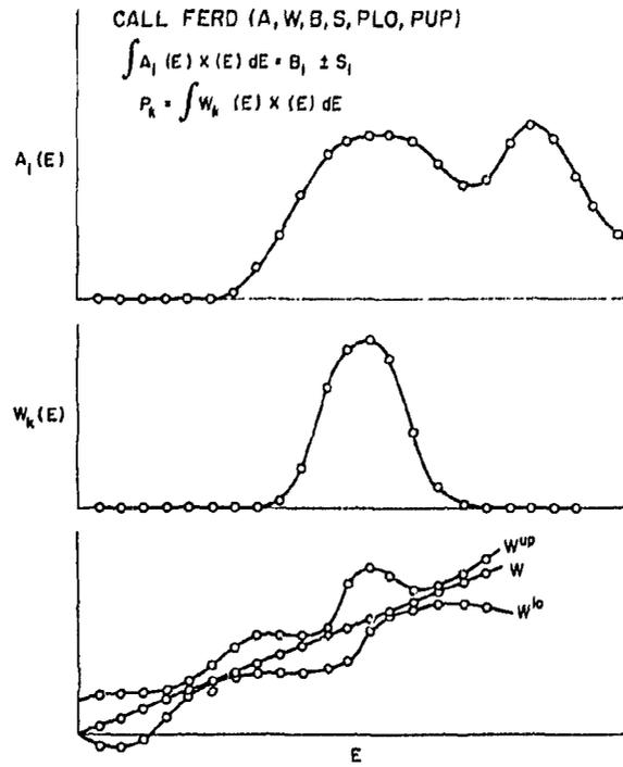
Fig. 7. Input-Output of FERD Algorithm
