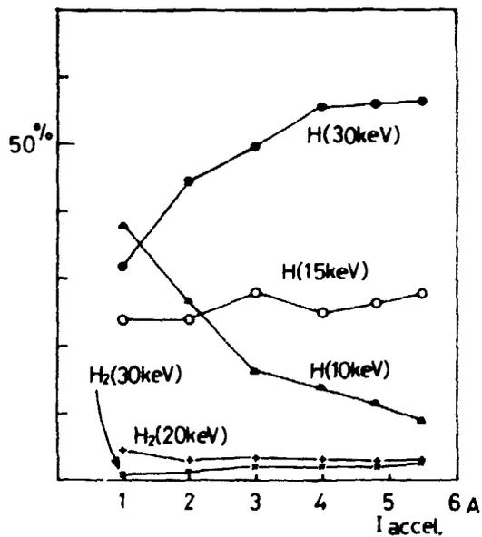
Fig. 1 Neutral power fractions at 30 kV extraction.
