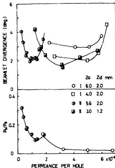
Fig. 5 Beamlet Divergence (deg) vs Perveance per Hole. Legend:  $z_a$   $z_d$  mm:  $\circ$  1.60 2.0,  $\square$  1.40 2.0,  $\bullet$  1.56 2.0,  $\blacksquare$  1.30 1.2.
