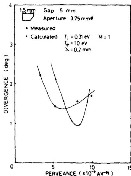
Fig. 6 Comparison of the measured beam divergence with calculated one.
