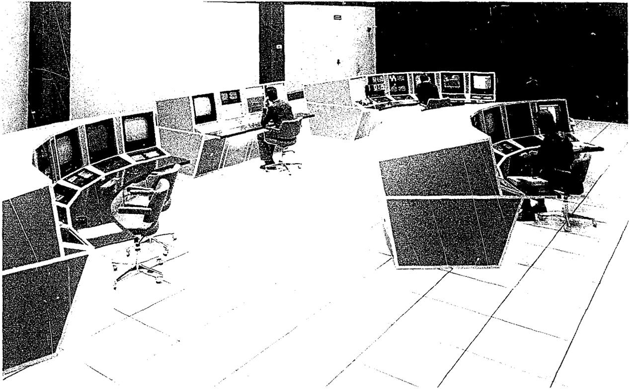
*The SPS Main Control Room. The accelerator may be operated from any of the three larger consoles, the smaller one being used for safety controls. (CERN 187.10.75)*
