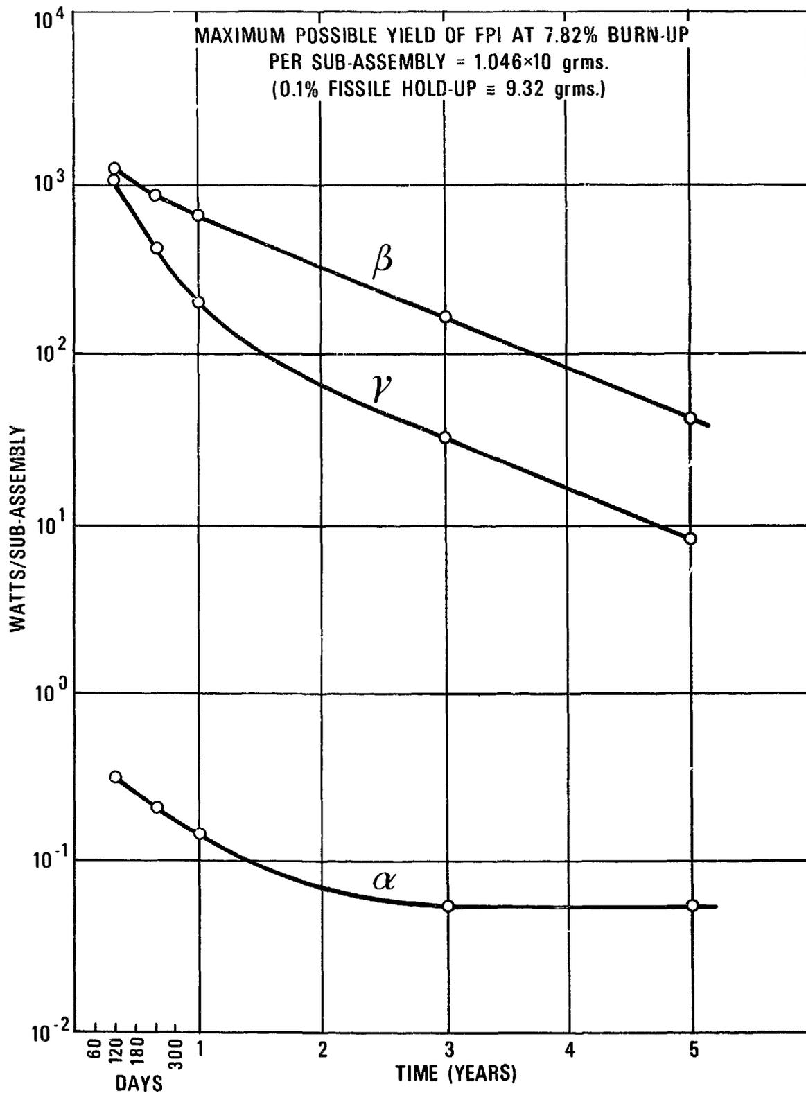
**Fig.5. HEAT OUTPUT OF MAXIMUM POSSIBLE YIELD OF FPI
