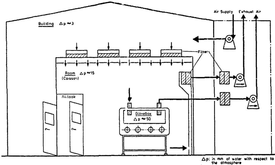
**Fig. 5:** Sketch of the Multiple Containments with Negative Pressure Zones
