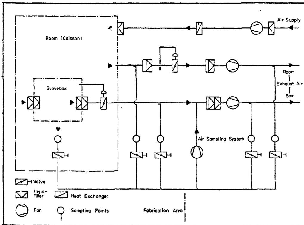
**Fig. 6:** Schematic Diagram of the Ventilation System
