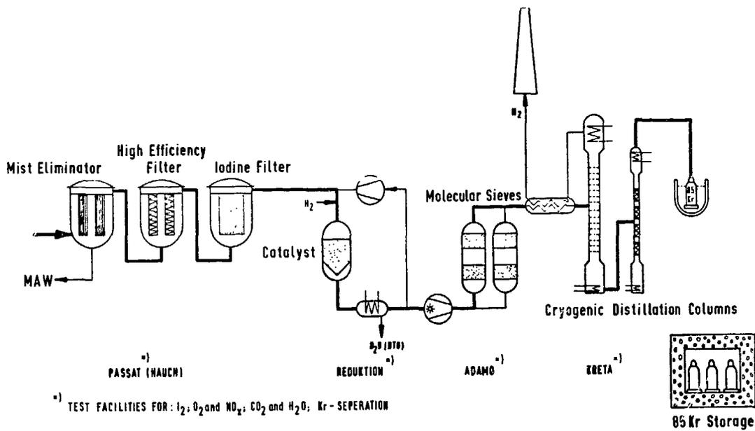
Fig. 4: Dissolver Offgas Cleaning System of a Reprocessing Plant
