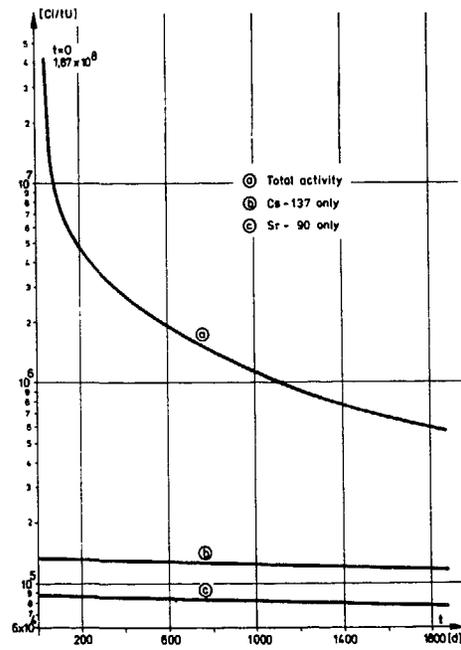
Fig. 2: Activity / tU as function of the fuel element cooling time
