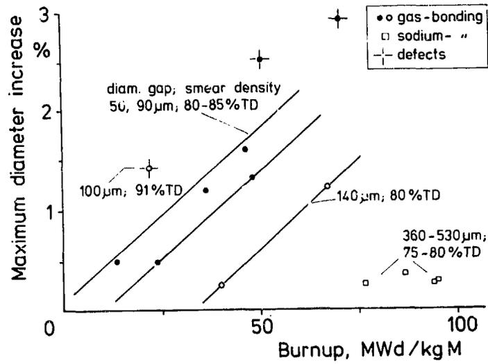
Fig. 3: Maximum cladding diameter increase of carbide fuel pins of different fuel density and bonding, after irradiation in thermal test reactors
