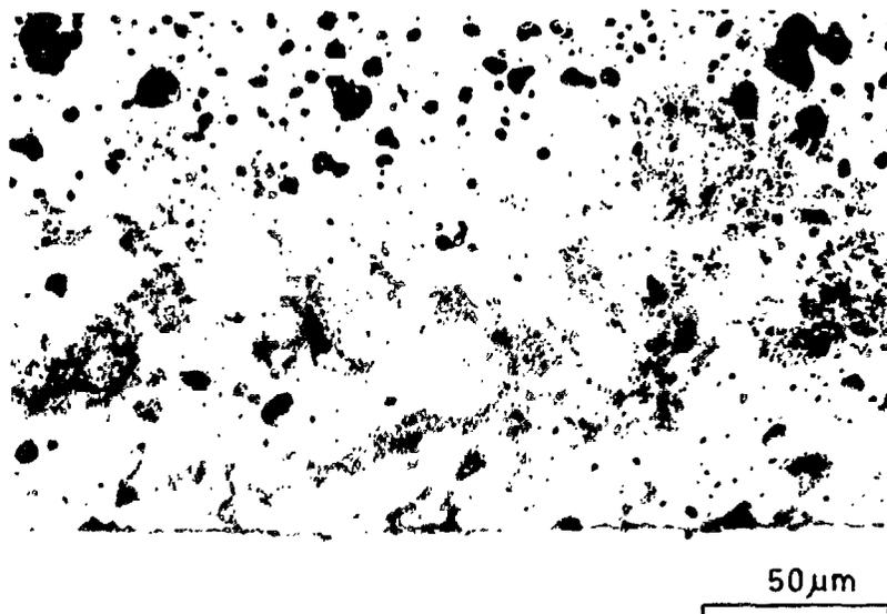
Fig. 5: Mixed oxide precipitates (dark phases) near the surface of mixed carbide fuel
