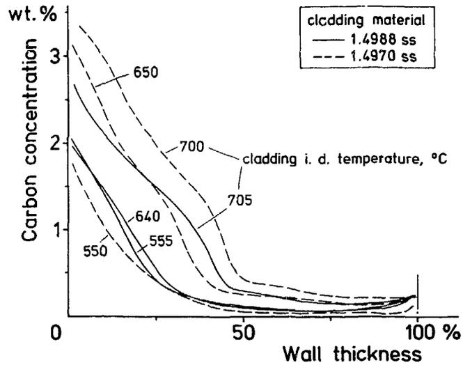
Fig. 8: Cladding carburization profiles in Na-bonded (U,Pu)C pins measured after DFR irradiation to about 5% burnup
