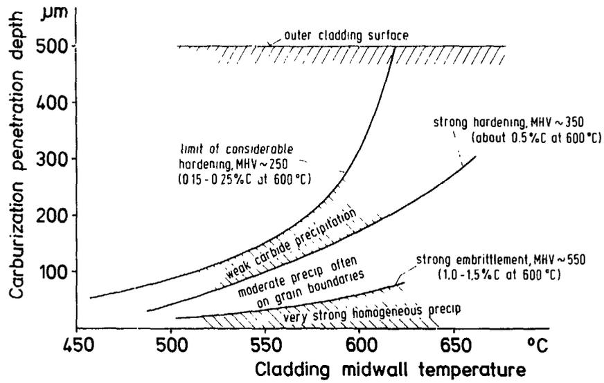
Fig. 9. Carburization of stainless steel cladding by high-carbon fuel (equivalent carbon content >5.15%) with Na-bonding in about 5000 h
