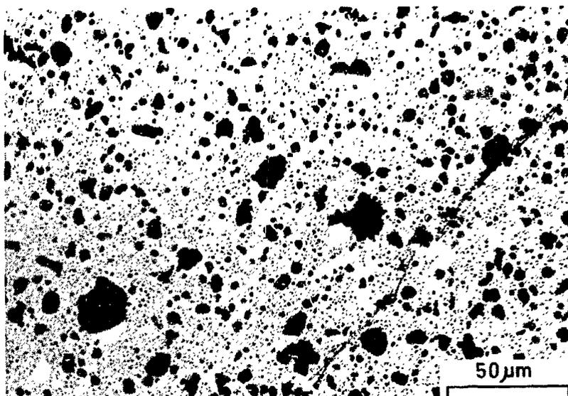
Fig. 6:  $(U,Pu)_2 \cdot (Tc,Ru,Rh)C_{v2}$  inclusions (bright phases) in hyperstoichiometric mixed carbide, burnup 7%
