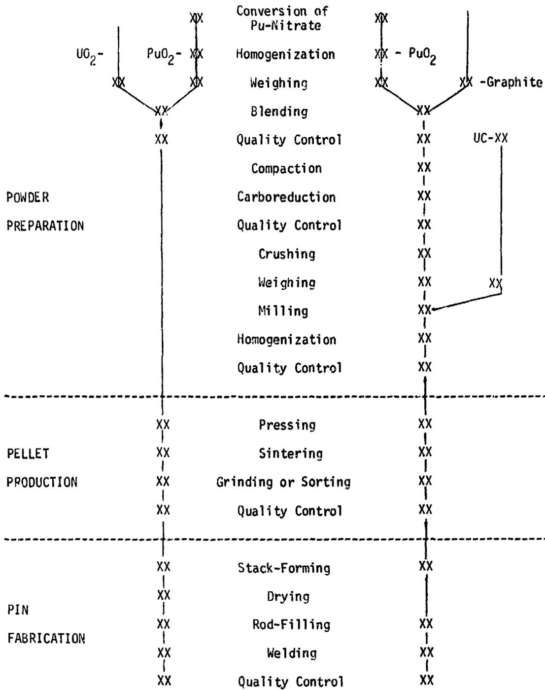
Fig. 2: Fabrication flow sheets for mixed (U,Pu) oxide and mixed (U,Pu) carbide
