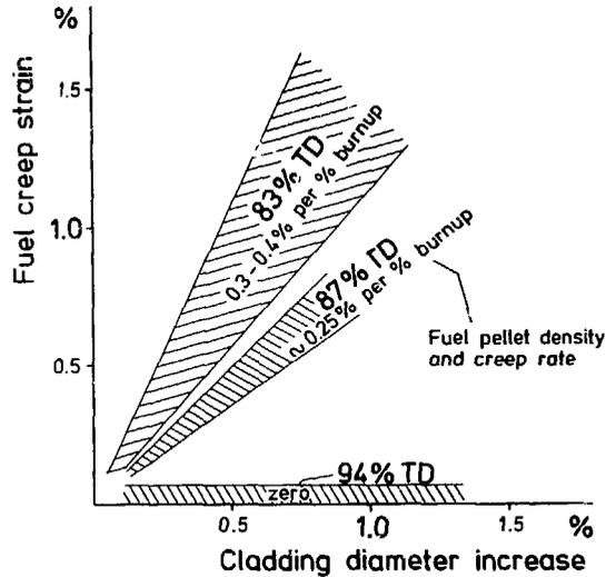
Fig. 10: Correlation of cladding strain and (U,Pu)C irradiation creep dependent on fuel density, under thermal test reactor irradiation
