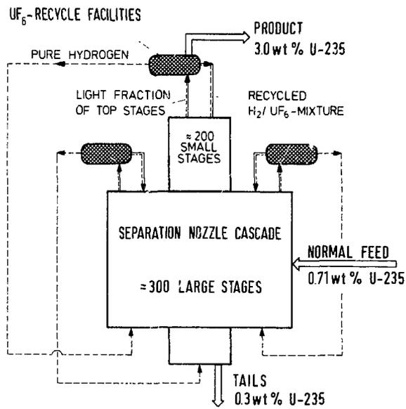
Fig. 5: Schematic representation of a separation nozzle cascade with UF<sub>6</sub> recycle facilities.
