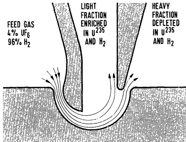
Fig. 1: Cross section of the separation nozzle system used in the commercial implementation of the process.
