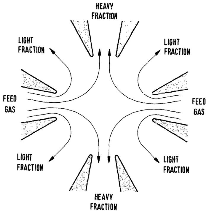
Fig. 7: Cross section of a separation nozzle system with opposed gas jets. /5/.
