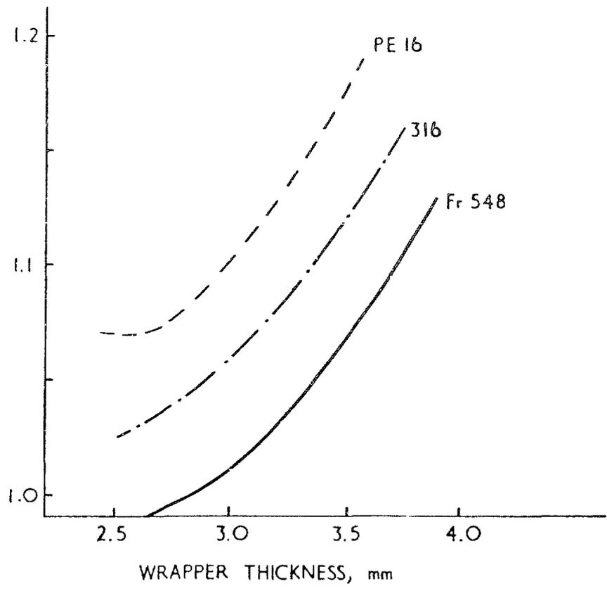
FIG. 2. RELATIVE URANIUM DEMAND AS A FUNCTION OF WRAPPER THICKNESS & MATERIAL
