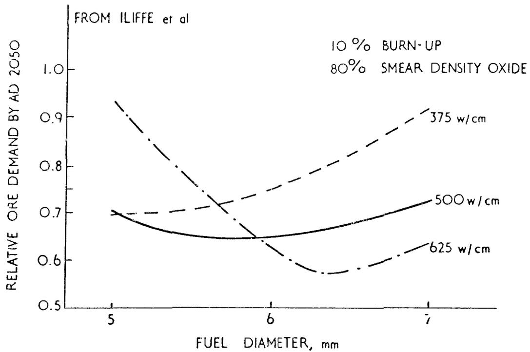
FIG. I. URANIUM UTILISATION AS A FUNCTION OF OXIDE PIN DIAMETER AND LINEAR RATING
