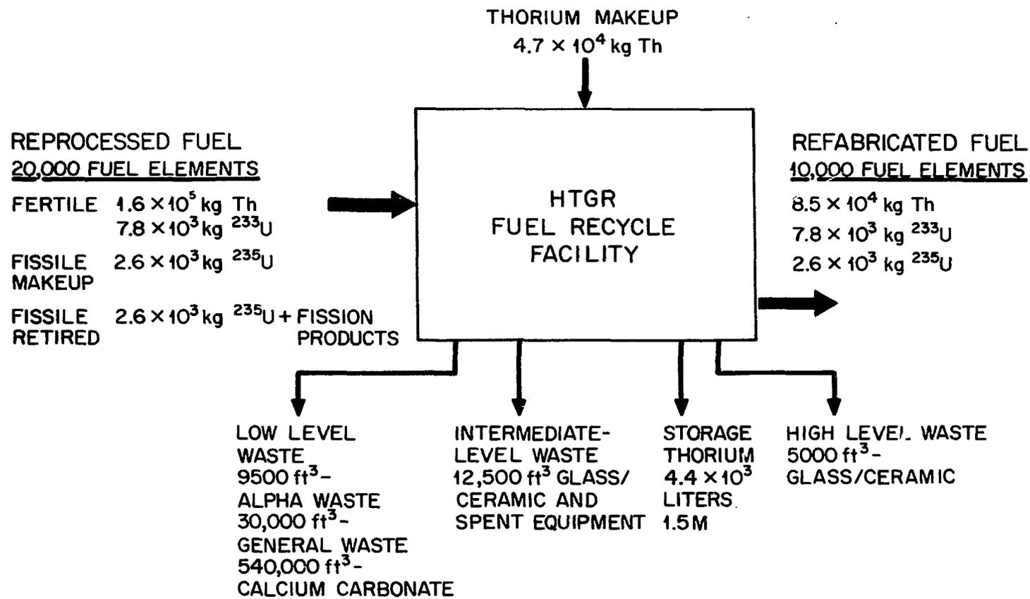
Fig. 5. Nominal Annual Materials Flow for a Central HTGR Fuel Recycle Facility.
