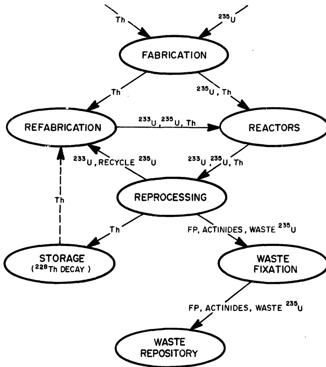
Fig. 4. Operations and Materials Flows in the HTGR Th-<sup>233</sup>U Fuel Cycle.
