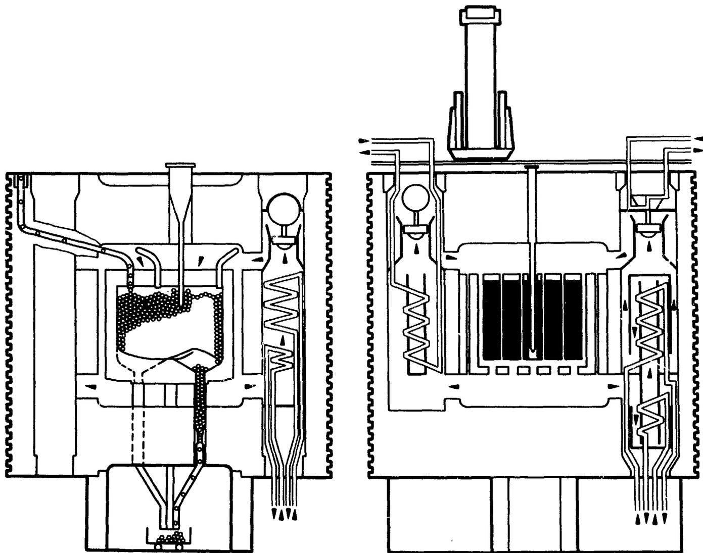
Fig. 3. Two Typical HTGR Designs. [Ref: H. Oehme, "Comparative HTGR Designs," pp. 72-91 in *Gas-Cooled Reactors: HTGR and GCFBR*, Gatlinburg, Tennessee, May 7-10, 1974, CONF-740501.]
