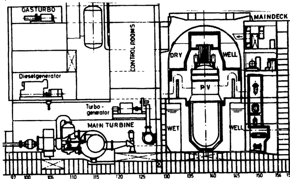
Fig. 5: NCS-80, Reactor and Machinery Space
