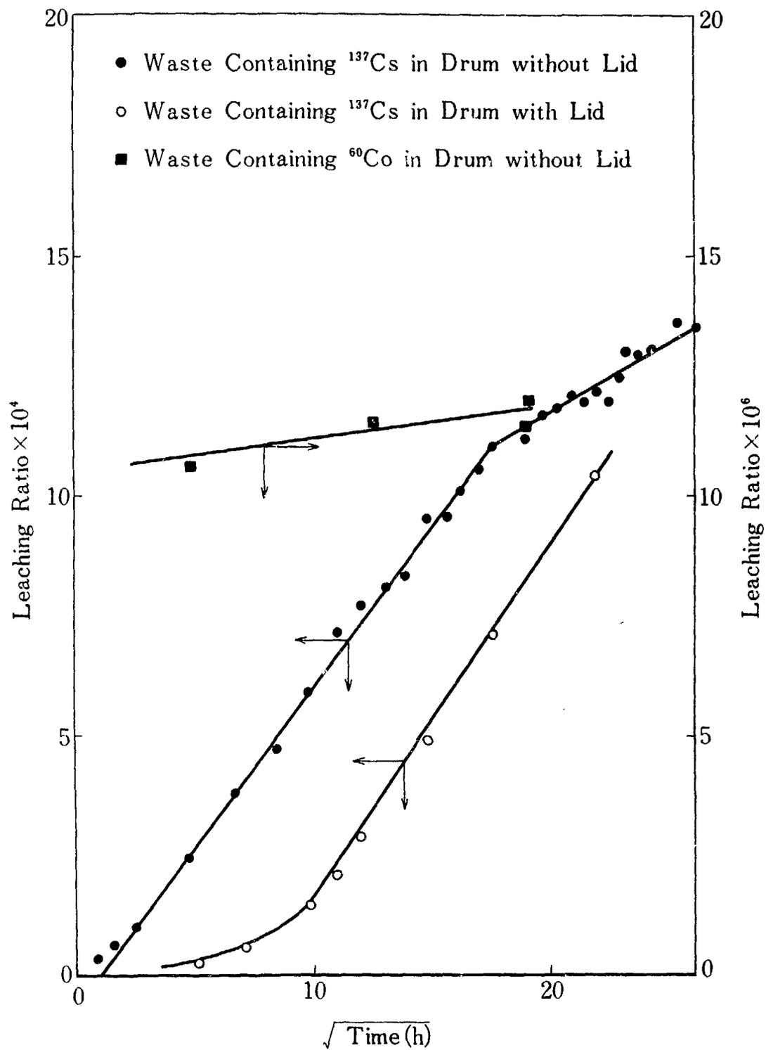
Fig. 1. Leaching under High Pressure from Low-Level Waste—Cement Composite Solidified in 200 l Drum
