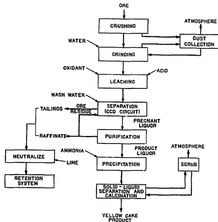
**FIGURE 2. URANIUM MILL - ACID LEACH PROCESS SIMPLIFIED BLOCK FLOW DIAGRAM**
