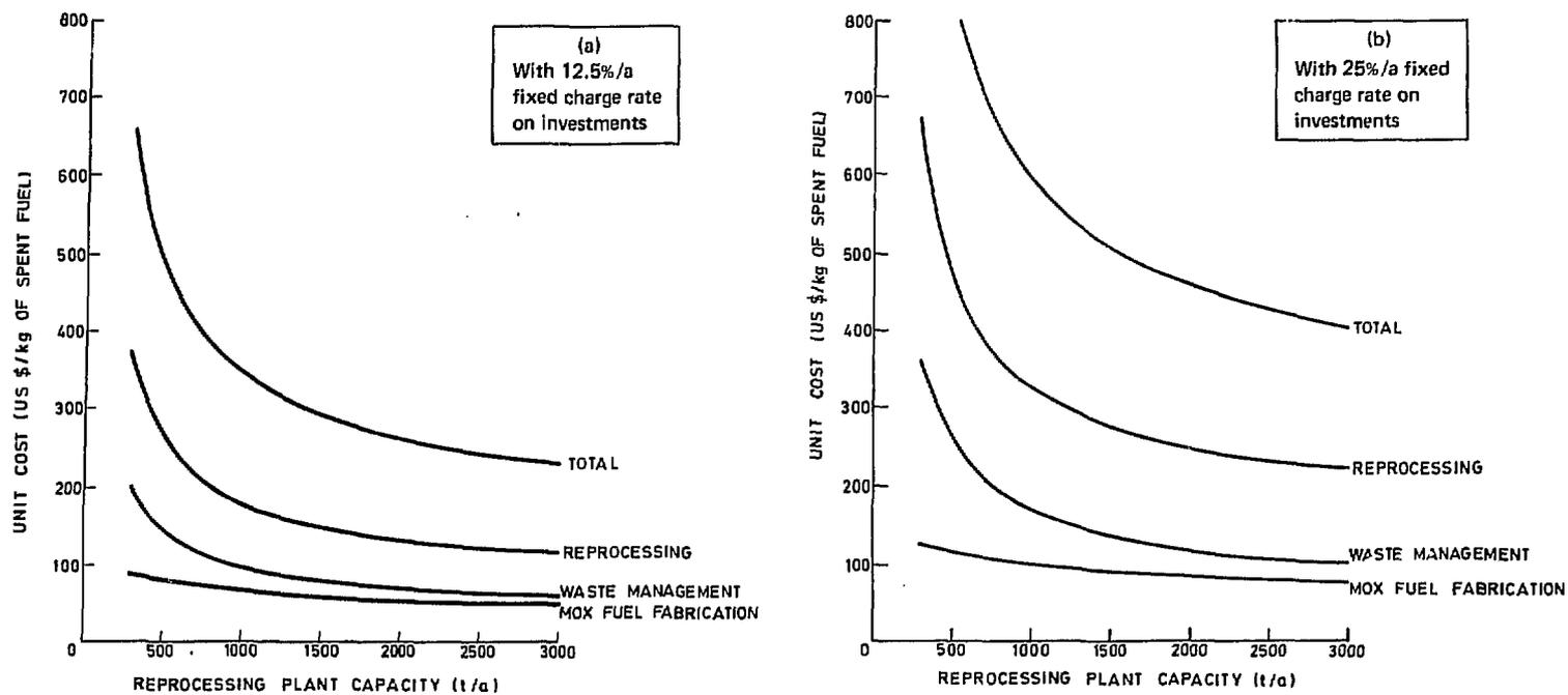
Fig.5. Economy-of-scale effects on unit costs of reprocessing, MOX fuel fabrication and waste management (all costs are per kilogram of spent fuel reprocessed).
