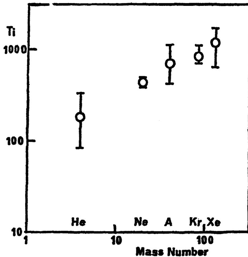
Fig. 3, Mass Dependence of Ion Temperature of Hot Component of Turbulently Heated Plasma Ions.
