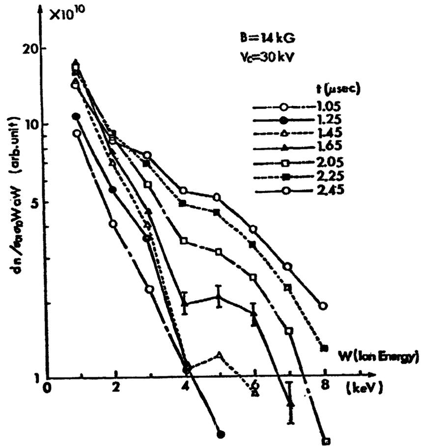
Fig. 2. Temporal evolution of the high energy part of the ion energy spectrum. The charging voltage of the capacitor for heating  $V_c$  is 30 kV.
