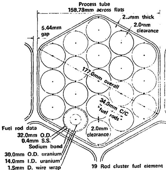
**FIGURE 6.** Fuel Assembly Cross Section (Full Size)
