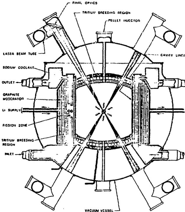
**FIGURE 2.** Side View of a Conceptual Laser Fusion Hybrid Reactor
