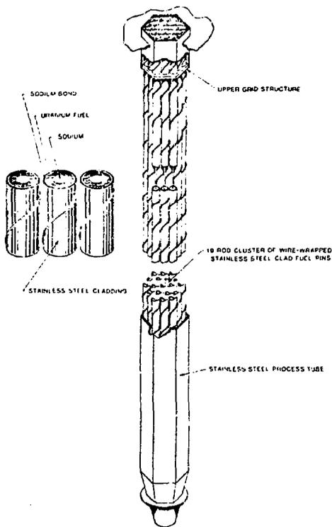
FIGURE 7. Fuel Element and Process Tube Configuration
