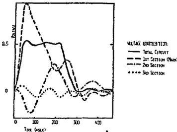
Fig. 6 Contributions to load voltage for a 3 stage PFN
