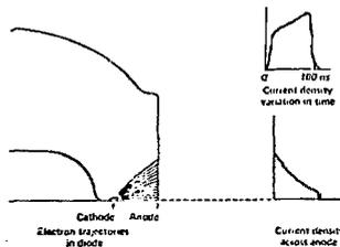
Fig. 8 PFBS e gun characteristics
