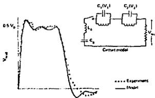
Fig. 7 Load voltage for 3 stage Vigil PFN
