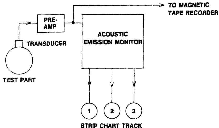
FIGURE 2 - ACOUSTIC EMISSION EXPERIMENTAL SET-UP
