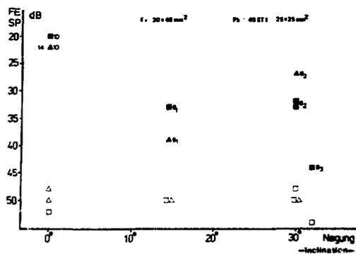
Fig. 5: Flaw echo (FE) and noise level (SP) values for reflectors of the same size
