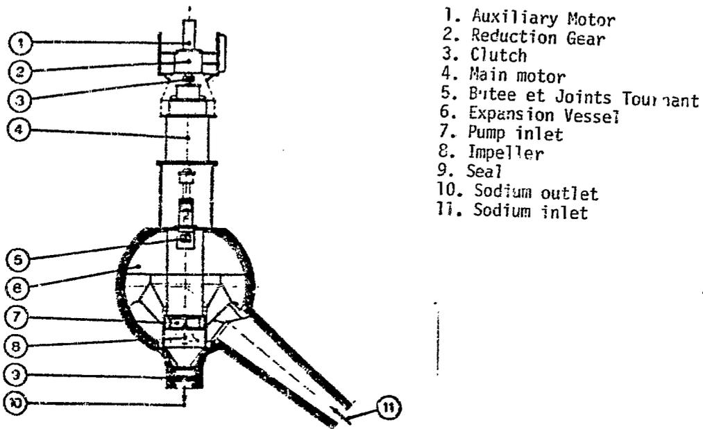
Fig. 3. Expansion Reservoir and Secondary Pump
