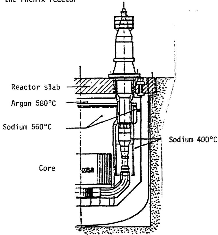
Fig. 2. Positioning in the Reactor of a Phenix Type Pool Pump
