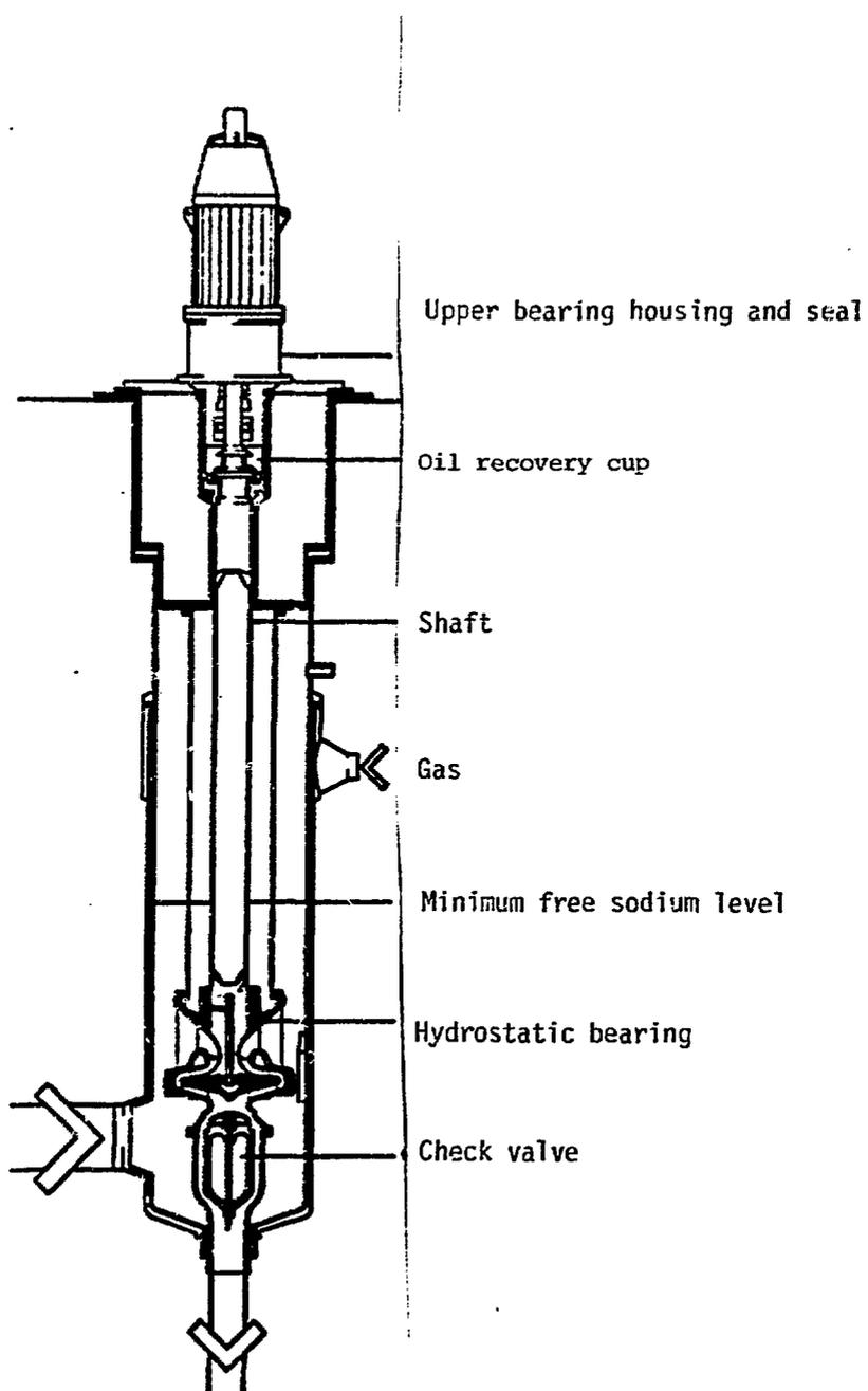
Fig. 1. Cross-section of a Rapsodie Type Primary Pump
