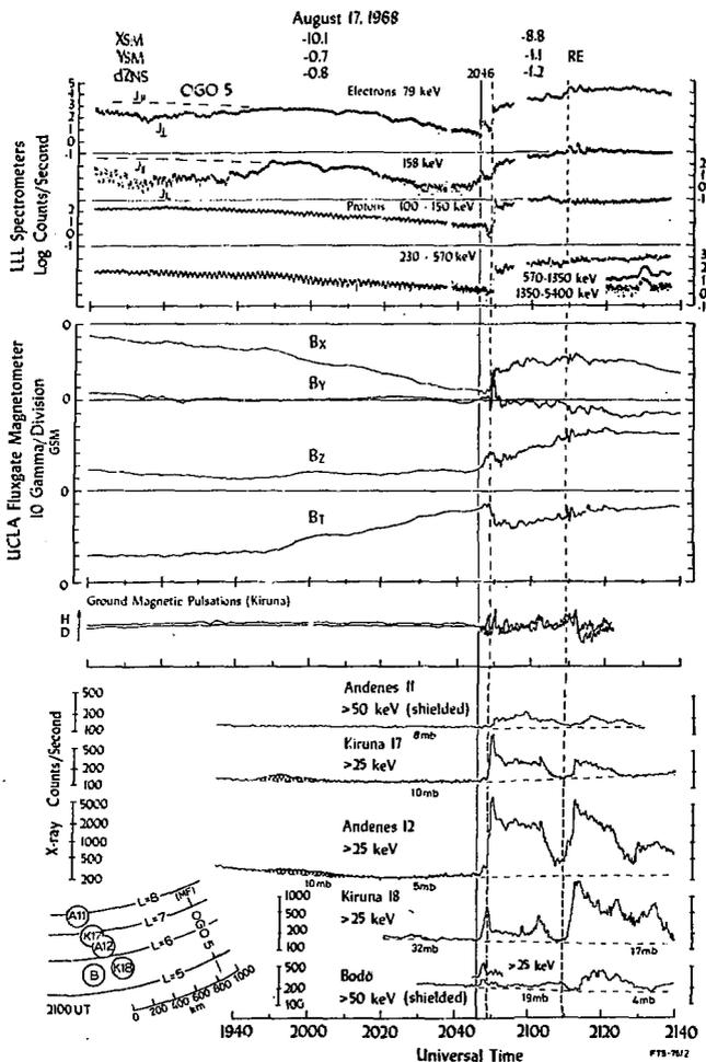
**Figure 5** Simultaneous observations in the nighttime plasma sheet by the OGO 5 satellite and near the earth's surface by a north-south chain of balloons. The ionospheric intersection of the field line through OGO at 2100 UT, estimated by field-line tracing according to the Mead-Fairfield model MF73Q, is indicated by MF in the bottom left diagram. Normalized parallel electron fluxes at OGO are based upon data from the UCLA particle experiment. (From Pytte and West, 1976).
