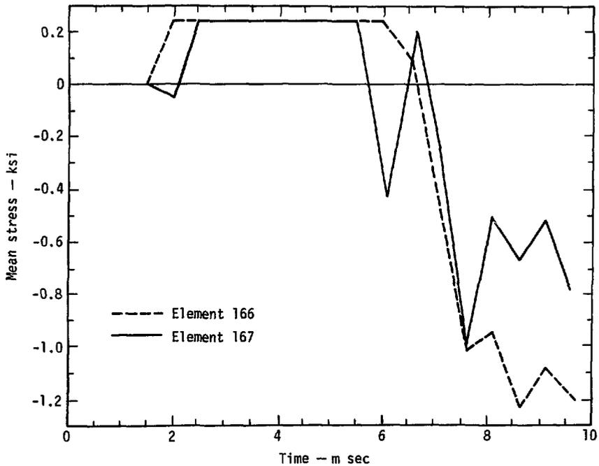
Fig. 27. A 12-in.-diam. pipe: mean-stress time histories (elements 166 and 167).
