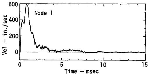
b) Test B2: Missile velocity = 275 fps
