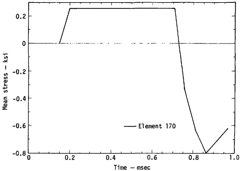
Fig. 29. A 12-in.-diam. pipe: mean-stress time histories (element 170).
