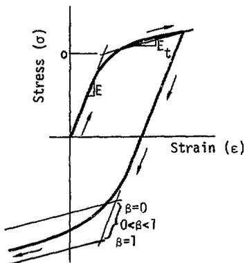
Fig. 3. Typical stress-strain behavior of a ductile metal bar.
