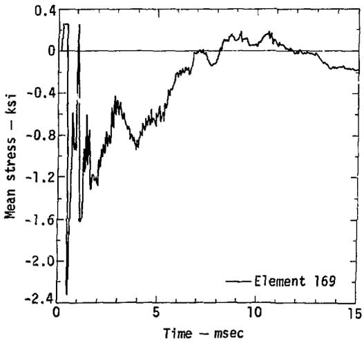
Fig. 13. Test 4F: mean-stress time histories (perimeter impact area).
