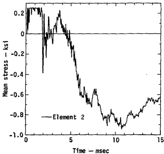
Fig. 10. Test 4F: mean-stress time histories (back-face elements).
