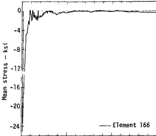
Fig. 12. Test 4F: mean-stress time histories (center of impact).
