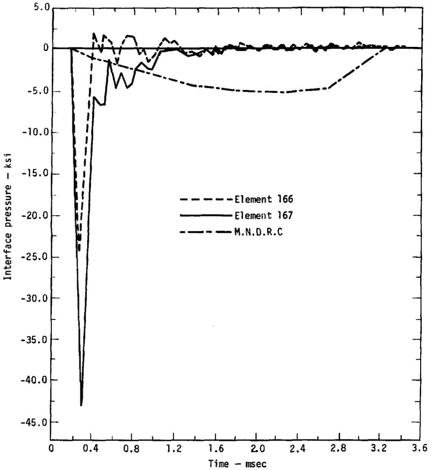
Fig. 22. Test A2: interface-pressure time histories.
