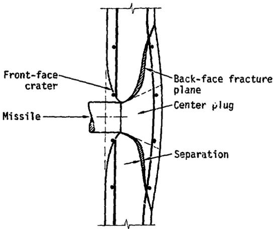
Fig. 2. Typical fracture planes<sup>8</sup> (impact velocity near threshold of scabbing).
