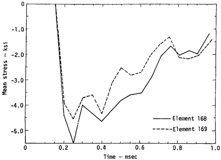
Fig. 28. A 12-in.-diam. pipe: mean-stress time histories (elements 168 and 169).
