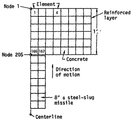
Fig. 9. Finite element mesh at the point of impact.
