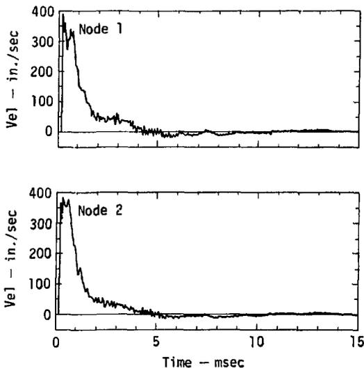
Fig. 11. Test 4F: velocity time histories (back-face nodes).
