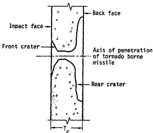
Fig. 1. Perforation of concrete due to tornado-borne missile.
