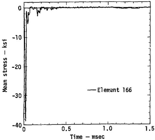
Fig. 16. Test 3F: mean-stress time histories (center of impact).
