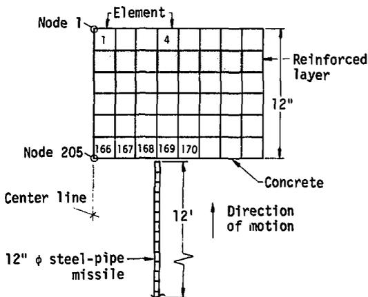
Fig. 25. Finite element mesh for deformable missile.
