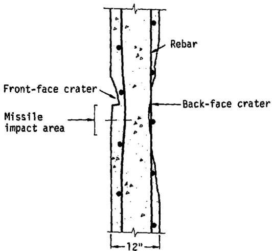
Fig. 8. Damage profile of Calspan Test No. 4F.
