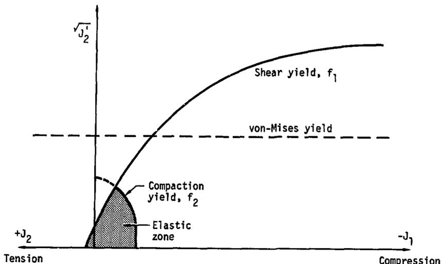
Fig. 7. Yield surfaces for concrete in  $\sqrt{J_2} - J_1$  space.<sup>21</sup>
