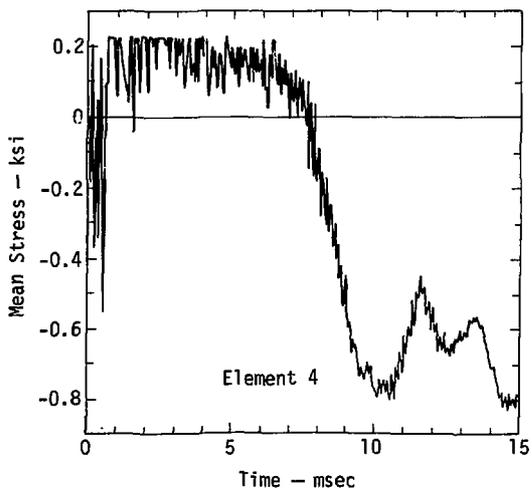
Fig. 14. Test 3F: mean-stress time histories (back-face nodes).
