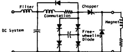
Figure 2. Chopper Schematic
