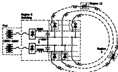
Figure 1. Functional layout of power supply with choppers
