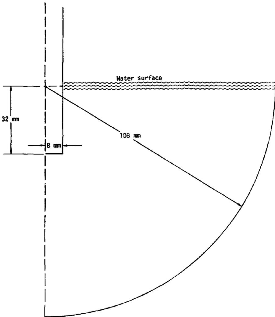
Fig. 1. Five-liter flask with submerged downcomer pipe.
