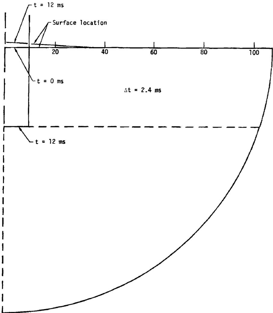
Fig. 4. Five-liter flask during pipe venting. Free surface location vs time.
