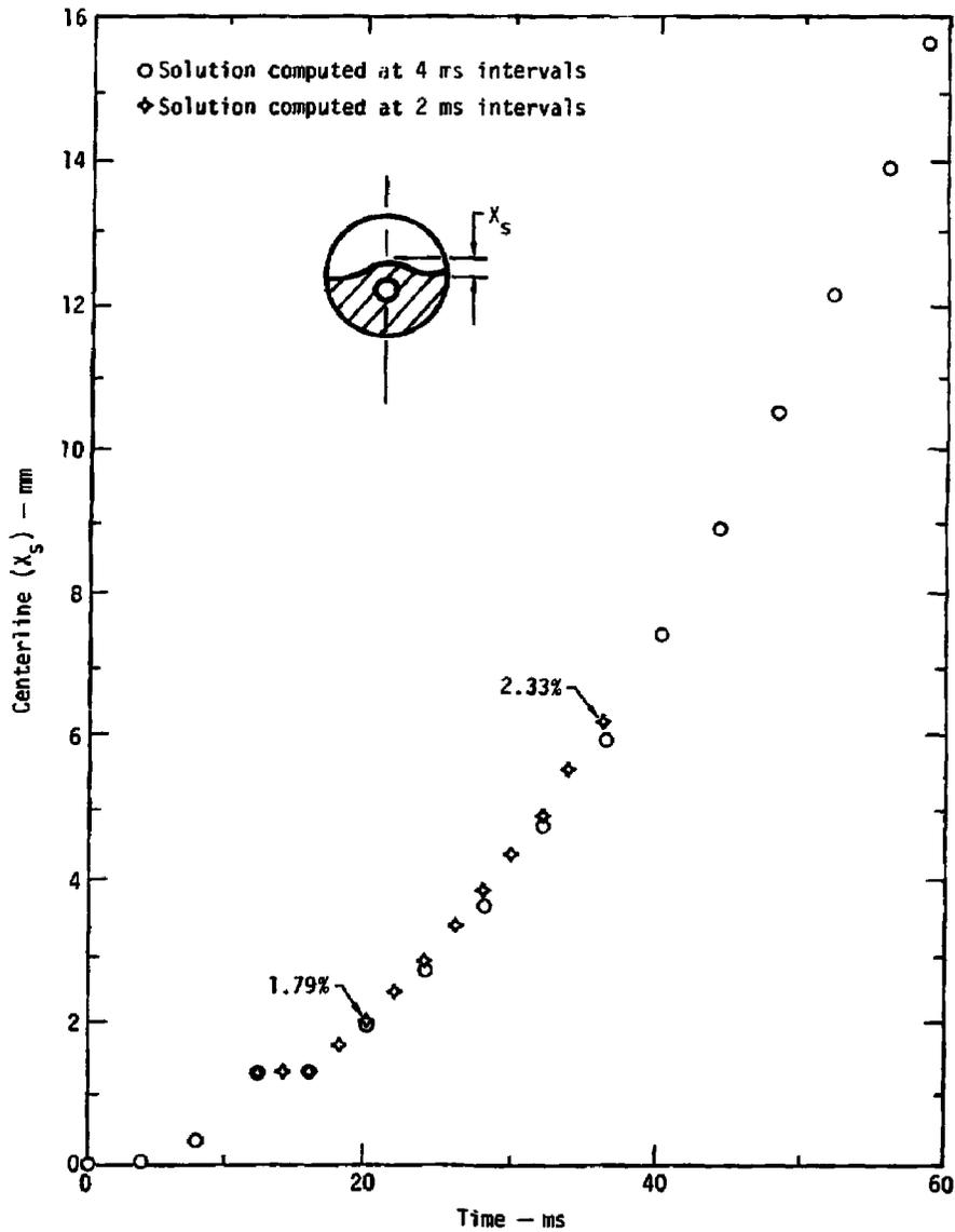
Fig. 6. Five-liter flask during bubble expansion showing the location of free surface centerline vs time.
