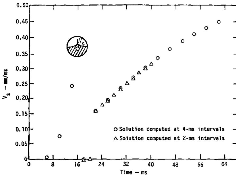
Fig. 5. Five-liter flask during bubble expansion showing centerline free surface velocity vs time.
