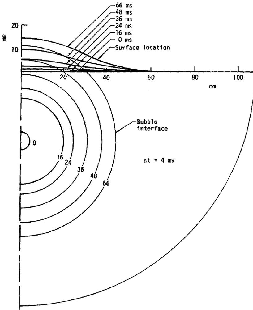
Fig. 7. Five-liter flask during bubble expansion showing bubble and free surface location vs time.
