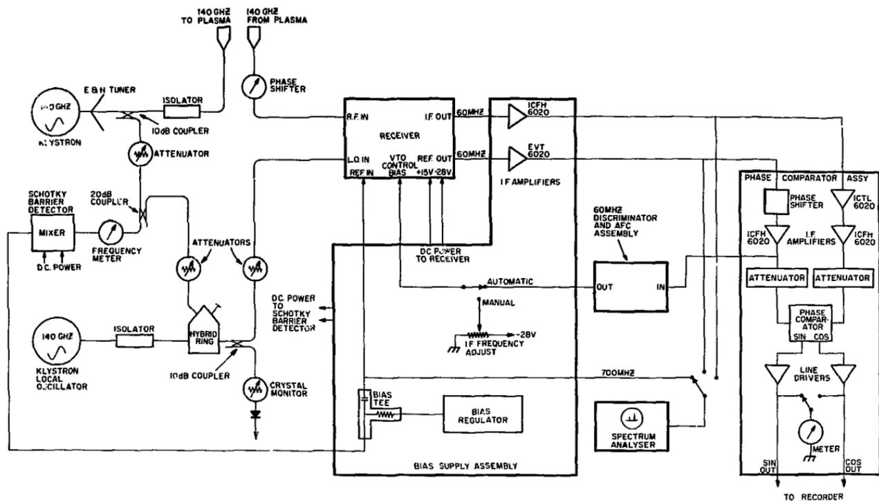
Fig. 1. Microwave interferometer phase detection circuits (Dwg. No. LEA 77-250164-00).
