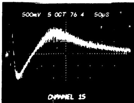
(a) Output during decay of laser-produced plasma.
