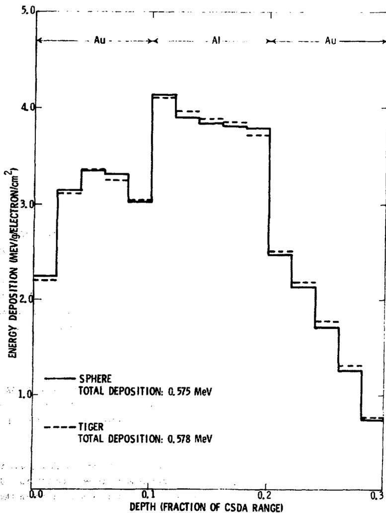
Figure 7. Comparison of electron energy deposition profiles calculated with the SPHERE and TIGER codes.
