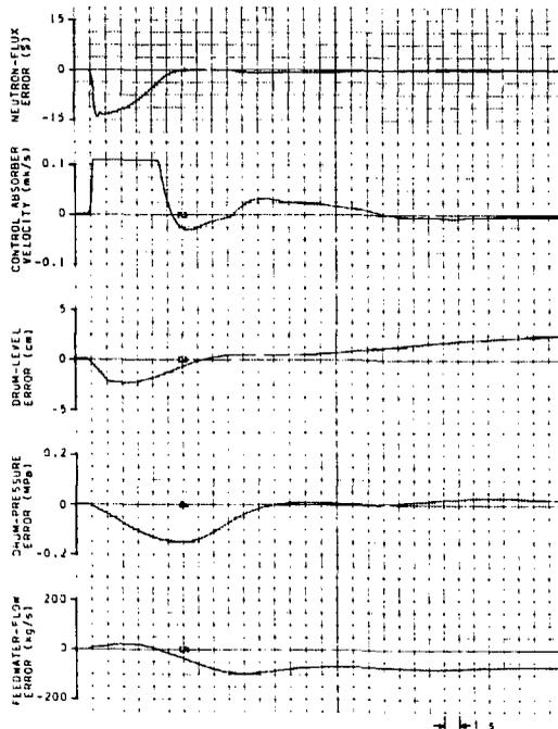
FIGURE 7 - TRANSIENT RESPONSE OF CANDU-BLW(PB)-1200 TO A FEEDWATER-HEATER FAILURE
