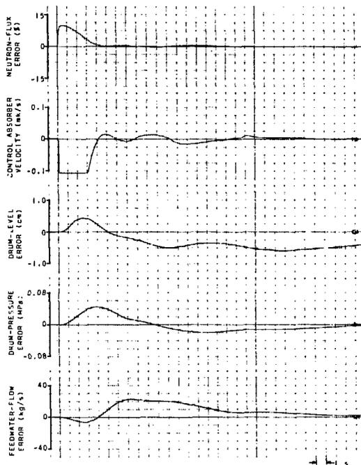
FIGURE 5 - TRANSIENT RESPONSE OF CANDU-BLW(PB)-1200 TO A 0.4 mk REACTIVITY STEP
