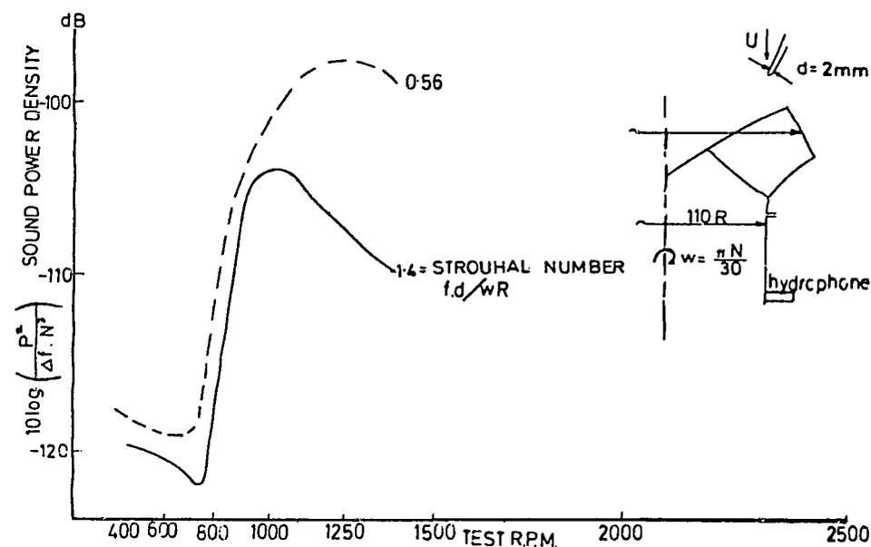
FIG1 INCEPTION OF CAVITATION NOISE IN PUMP AS SPEED IS INCREASED AT CONSTANT THROTTLE AND NPSH. P = THIRD OCTAVE SOUND PRESSURE (PASCAL), f = FREQUENCY,  $\Delta f$  = FREQUENCY BAND WIDTH (Hz) N = RPM.
