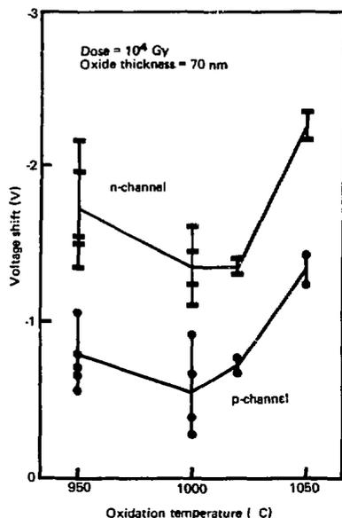
**Fig. 3** Radiation-induced voltage shifts are minimized if the gate oxide layer is grown at a temperature of about 1000°C.
