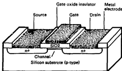
**Fig. 1** A CMOS integrated circuit consists of n-channel and p-channel MOS transistors combined on the same substrate. For simplicity, only the n-channel transistor is shown. The formation of a minority carrier channel that controls the on-off state of the switch is highly dependent upon the magnitude of the electric field at the Si-SiO<sub>2</sub> interface.
