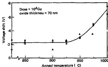
**Fig. 4** Radiation hardness is degraded if the postoxidation anneal temperature is greater than about 925°C.
