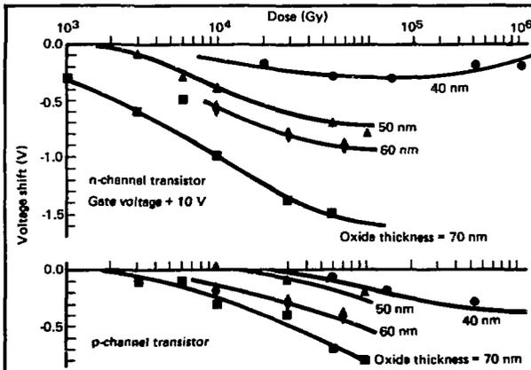
Fig. 2 The shift in turn-on voltage produced by a given radiation dose is reduced as the oxide layer is made thinner. Smaller voltage shifts imply harder devices. For a turn-on voltage of 2 V all these devices survive radiation exposures that are orders of magnitude greater than earlier commercial devices could tolerate.
