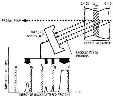
Fig. 2. Schematic of proton backscattering geometry (above) and graph of data showing abundance and depth-distribution of sample constituents (below). The "surface" relative to each element is indicated by the half-hashed lines. The horizontal axis, read from right to left, is proportional to depth for each element.
