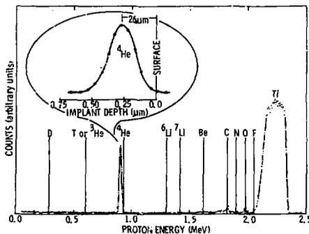
**Fig. 3.** This spectrum shows the number of protons backscattered with a given energy from a helium implanted foil. The excellent agreement between calculation (line) and analyzer data (points) is shown in the inset.
