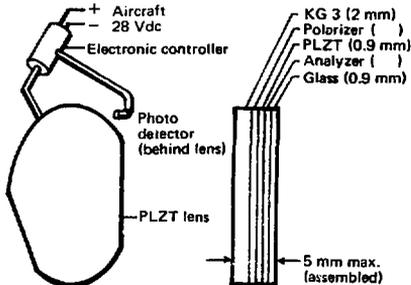
Fig. 3. Photo-optical feedback system and the laminated lens assembly.
