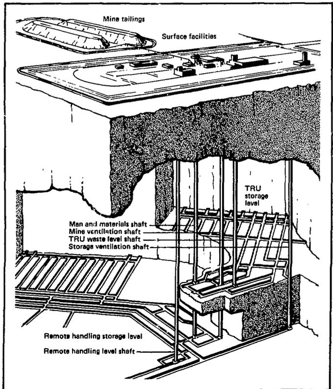
Fig. 2 The waste isolation pilot plant is a bi-level facility with storage at depths of 650 and 800 metres. Transuranic (TRU) contaminated wastes that can be contact handled are stored on the upper level; intermediate- and high-level wastes requiring remote handling are stored on the lower level.
