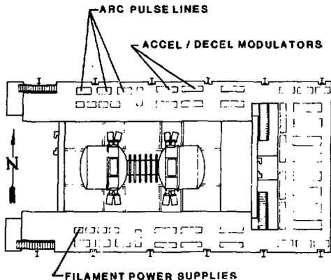
Figure 7. Second Tier Floor Plan.
