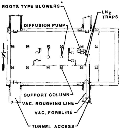
Figure 4. Pit Floor Plan.
