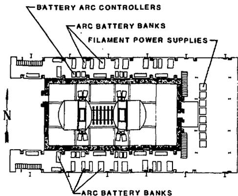
Figure 6. First Tier Floor Plan.
