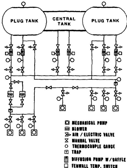
Figure 3. Vacuum Pumping Schematic.
