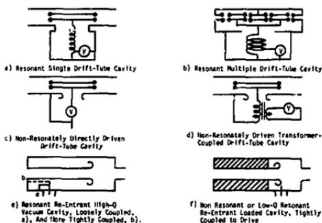
Fig. 2 - Resonant and Non-Resonant Structures
