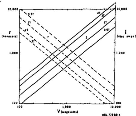
Fig. 1: Transport-limited current and pulse length versus voltage (see text for example parameters)
