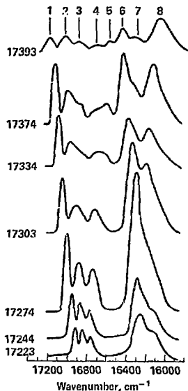
Fig. 3. Laser-excited fluorescence spectra of \text{Eu}^{3+} in 10\text{Li}_2\text{O} \cdot 90\text{B}_2\text{O}_3 glass at 2 K as a function of {}^7F_0 \rightarrow {}^5D_0 excitation energy ( \text{cm}^{-1} ).
