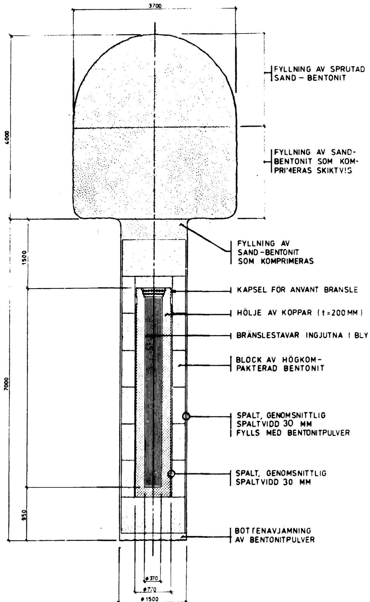
Fig.1a. Schematic picture of tunnel and deposition hole (VBB).
