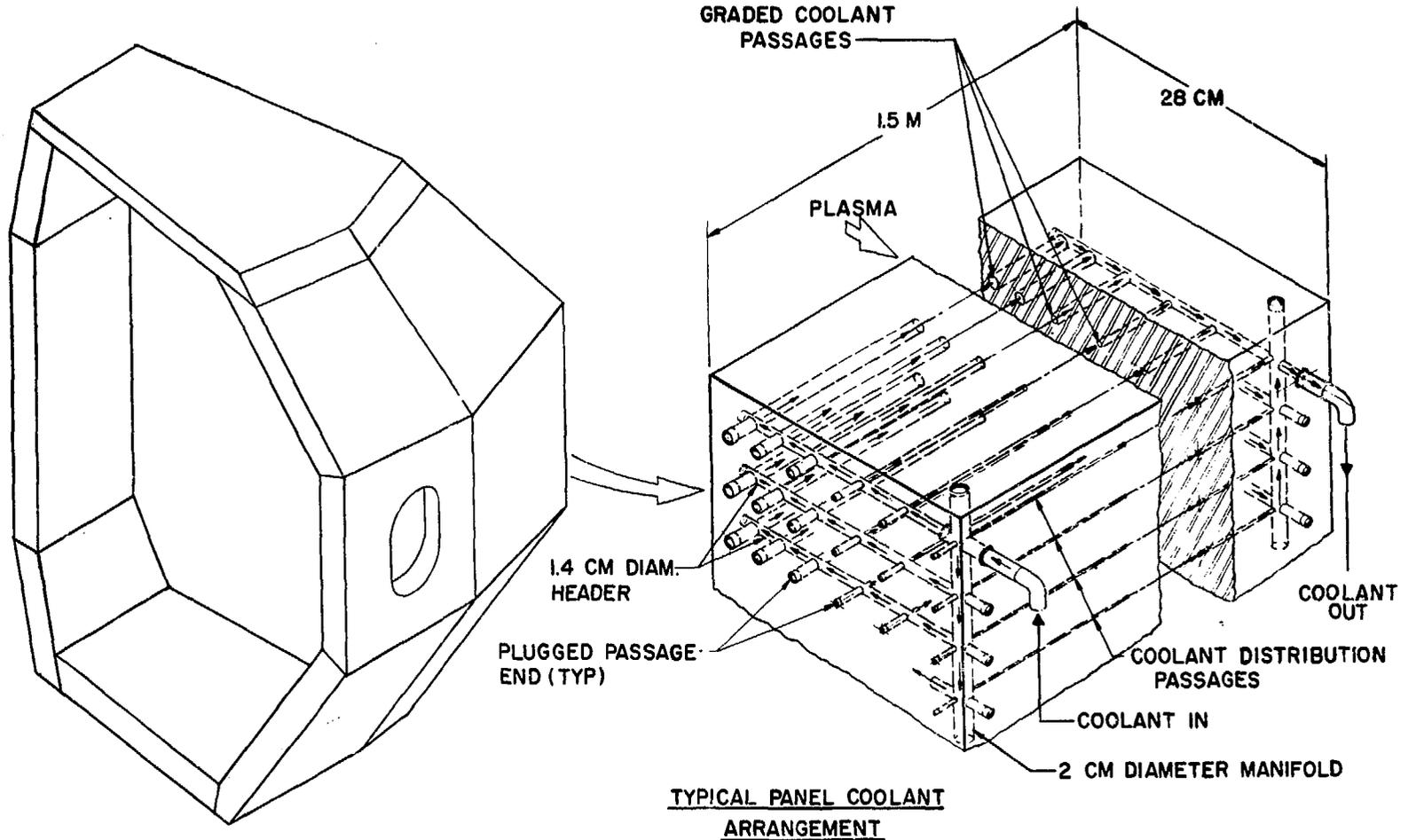
Figure II-2. Coolant Channel Arrangement for Stainless Steel Blanket Blocks Cooled with Water, Helium or Steam.
