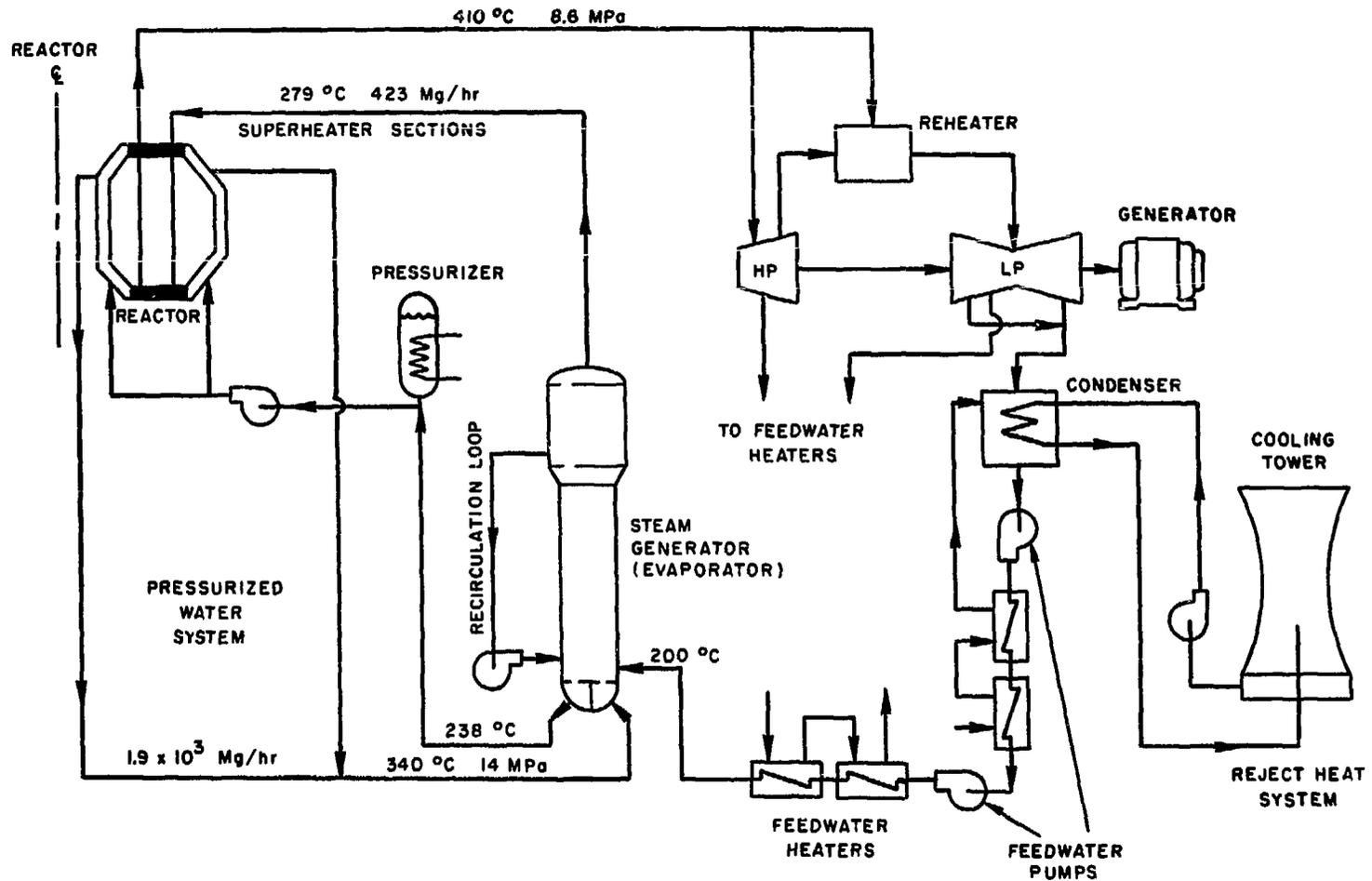
Figure II-4. Schematic of the EPR Coolant System.
