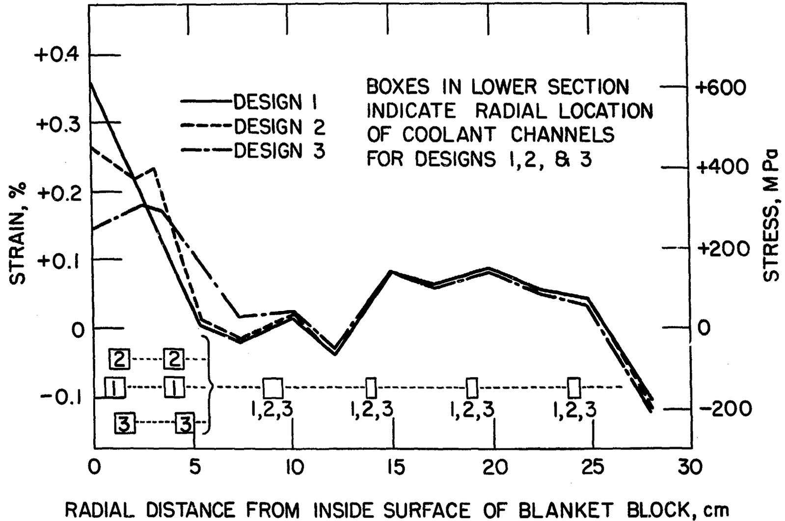
Figure II-3. Thermal Strain Distribution in Radial Direction for Various Channel Arrangements.
