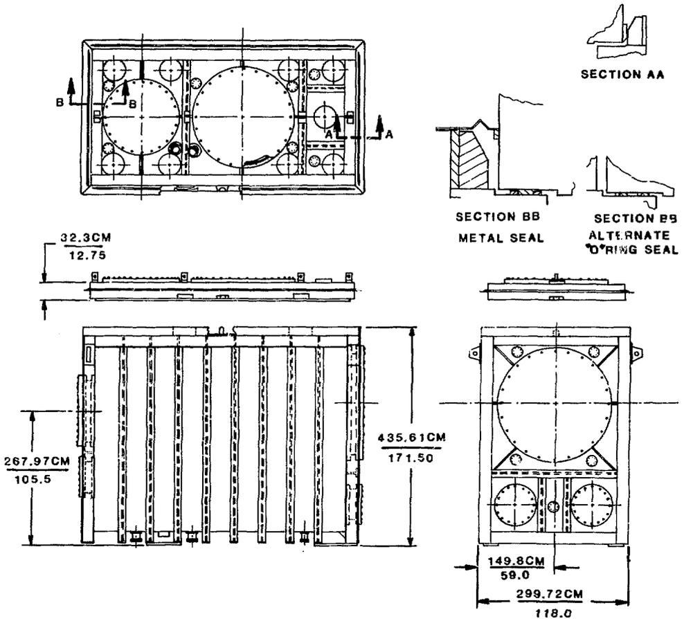
Figure 5. TFTR - NEUTRAL BEAM LINE VACUUM VESSEL
