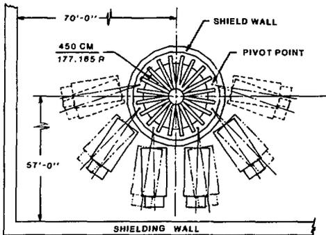
Figure 1. TFTR Neutral Beam Line Locations.
