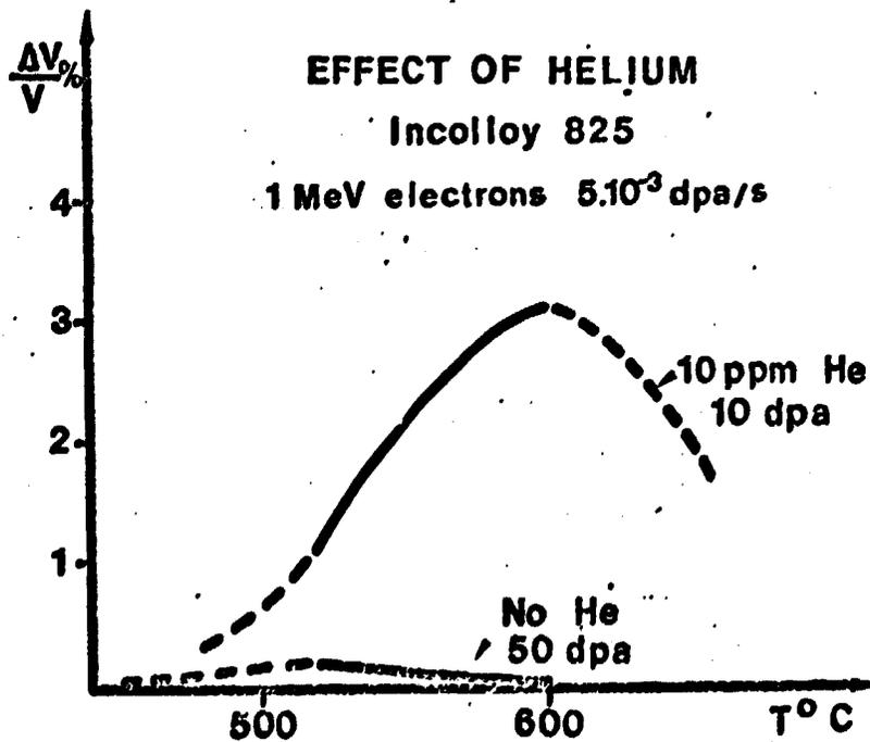
Fig. 3 - Effect of helium preinjection on swelling of Incolloy 825
