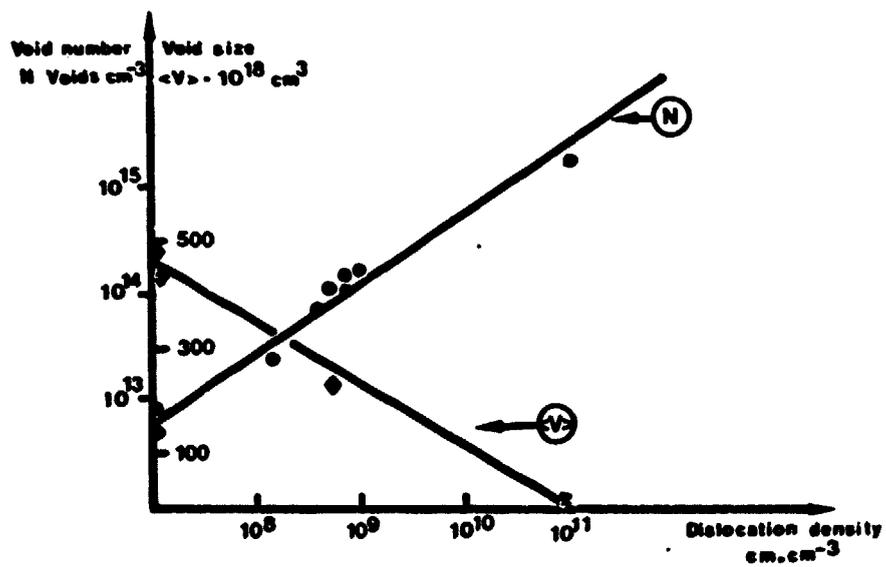
**Fig. 7** - Correlation between void number and size and preexisting dislocation density.
