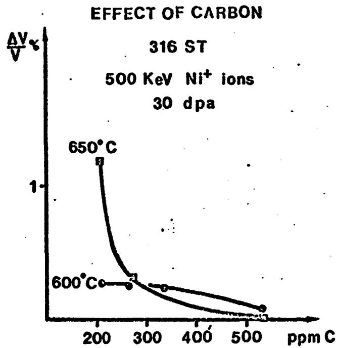
Fig. 12 - Temperature dependence of the effect of carbon on swelling of 316 steel.
