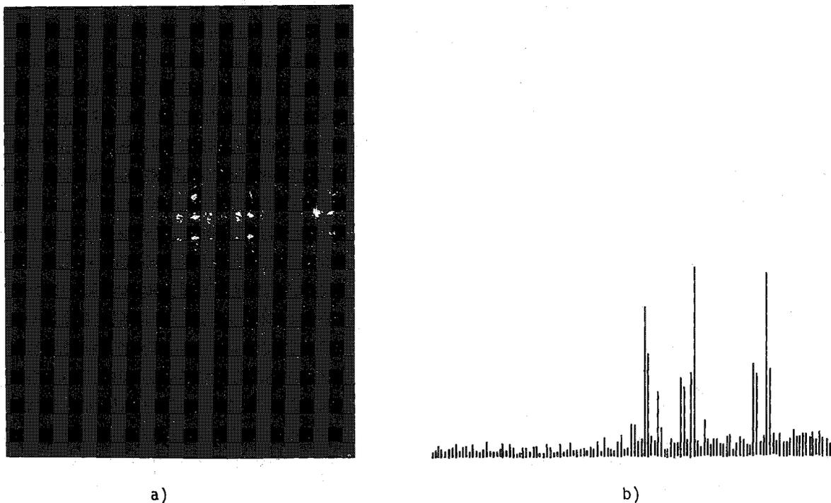
Fig. 3 a) The neutron image of three holes in a cadmium sheet. Each of the small spots is a hole in the drift space, spaced at 1 mm.
