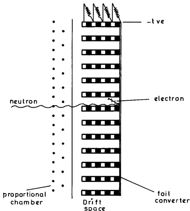
Fig. 1 The basic detector
