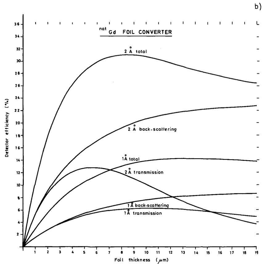
Fig. 2 a) Theoretical detection efficiencies for gadolinium-157
