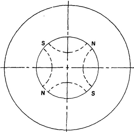
Fig. 3. Cylindrical Permanent Quadrupole Magnet
