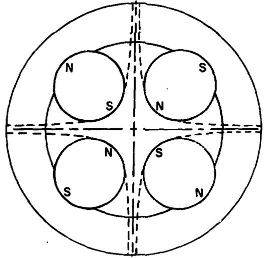
Fig. 7. Circular Pole Permanent Quadrupole Magnet
