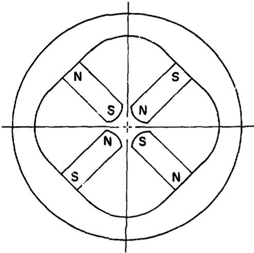
Fig. 5. Circular Truncated Pole Permanent Quadrupole Magnet
