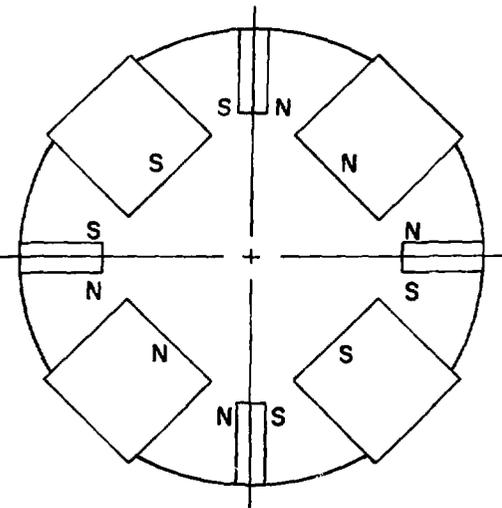
Fig. 4. Rectangular Pole Permanent Quadrupole Magnet
