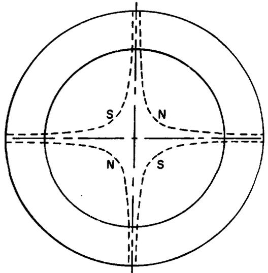
Fig. 1. Ideal Quadrupole Magnet
