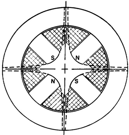
Fig. 2. Conventional Quadrupole Magnet
