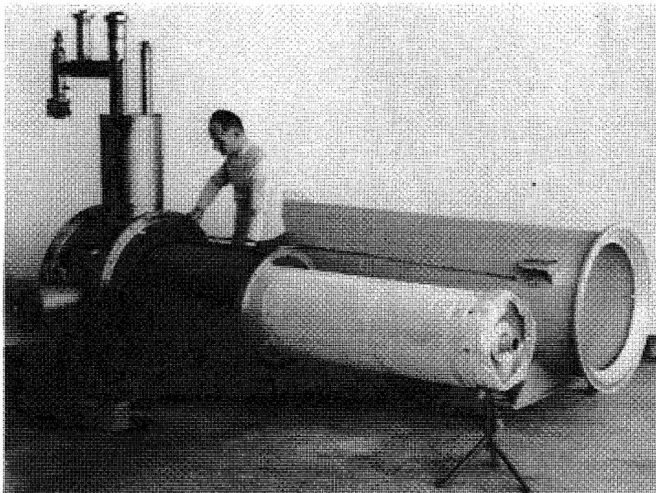
Fig. 16 Trial assembly showing super-insulated helium vessel, radiation shield, and vacuum tank
