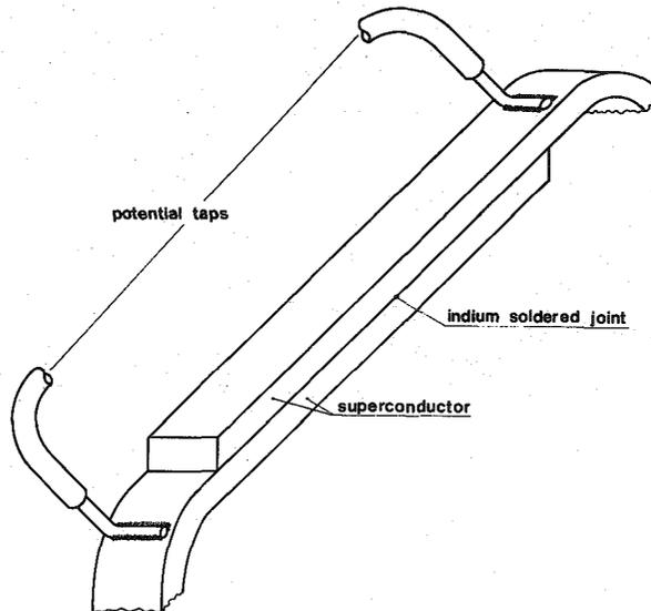
Fig. 11 Detail of inter-layer connection
