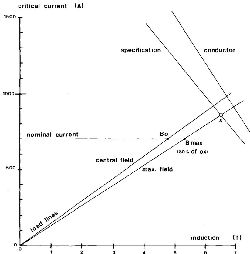
Fig. 2 Critical current -- field characteristics of composite conductors with magnet load lines
