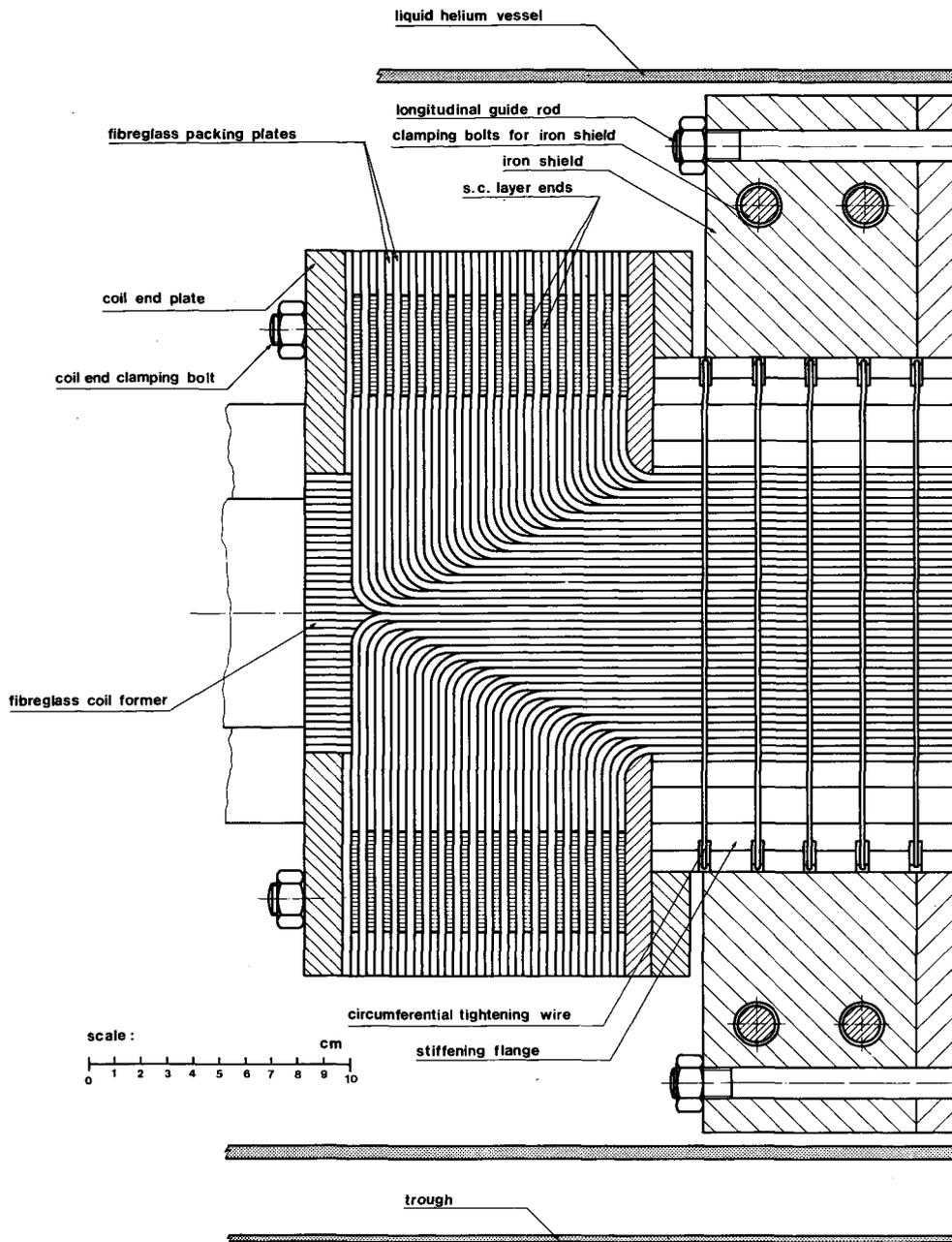
Fig. 3b Longitudinal section through coil end
