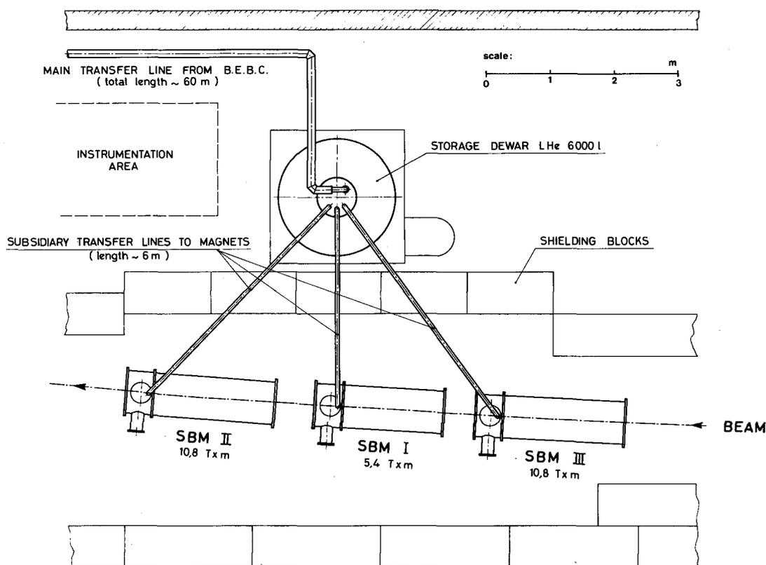
Fig. 1 Arrangement of magnets in beam line
