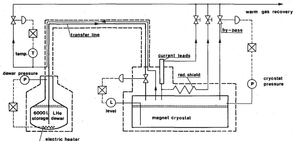
Fig. 19 Simplified helium flow scheme
