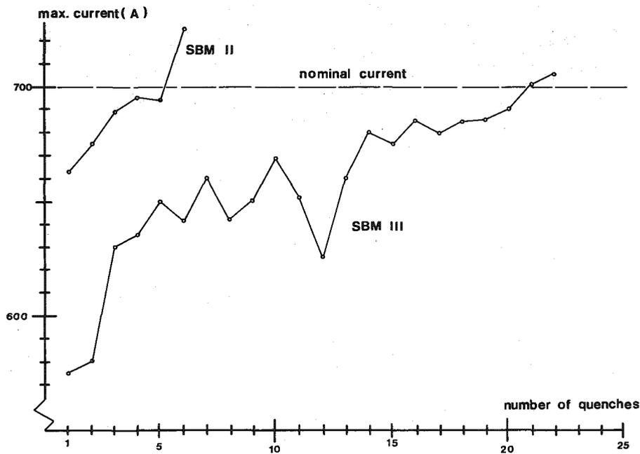
Fig. 14 Training curves; current versus number of quenches
