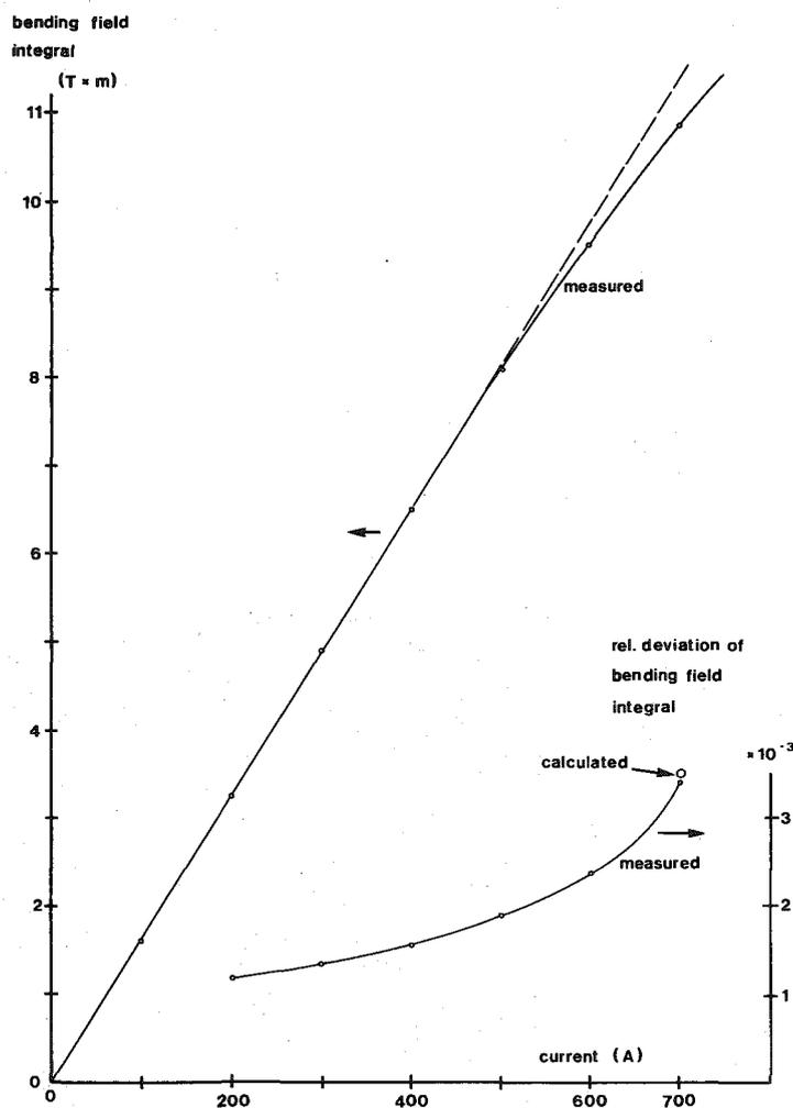
Fig. 21 Magnet calibration curve and field integral inhomogeneity versus current
