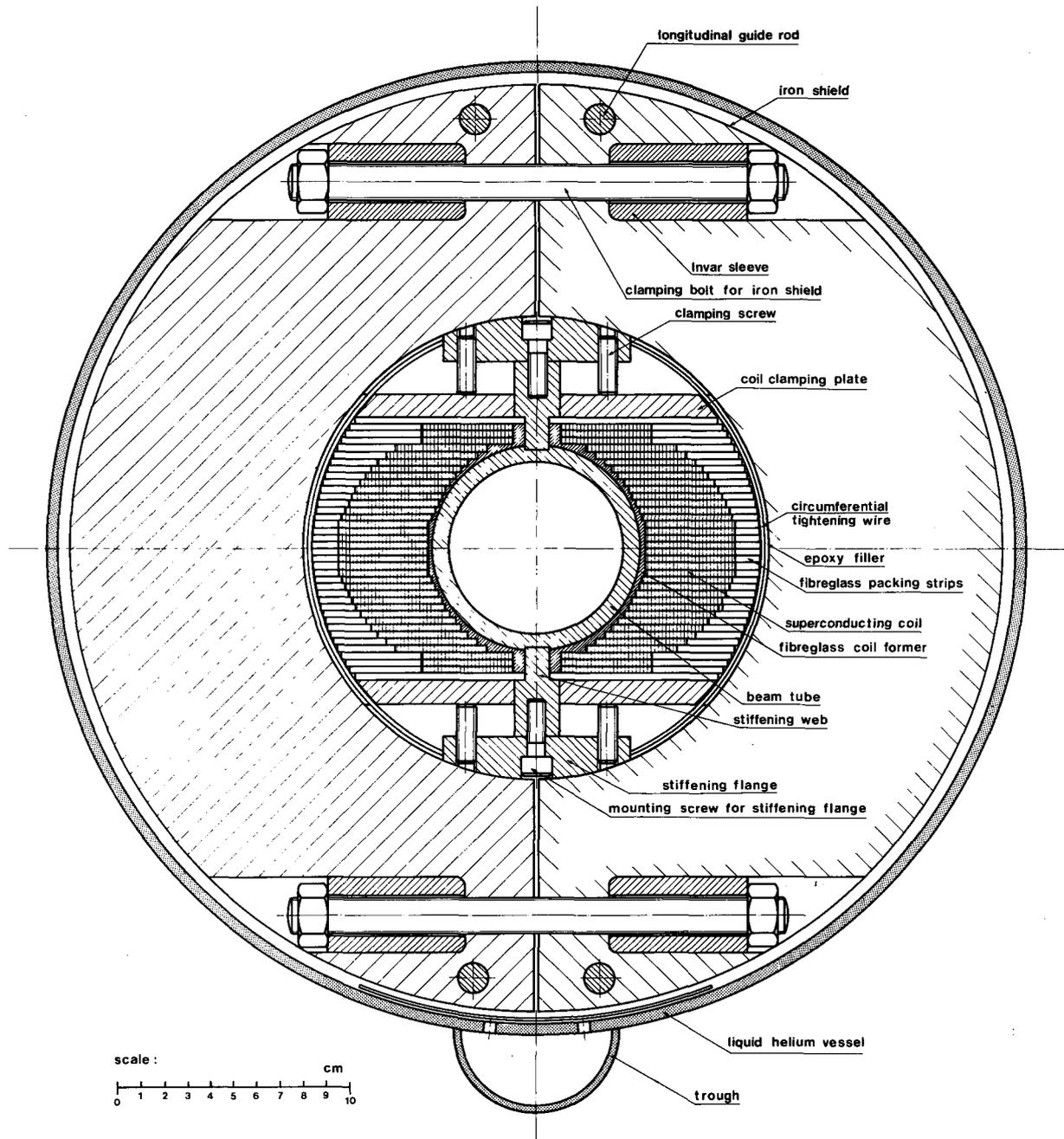
Fig. 3a Typical cross-section through straight part of magnet
