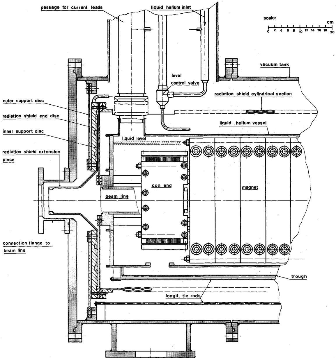
Fig. 15 Typical longitudinal cross-section through cryostat end
