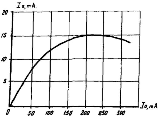
Fig. 5 Limiting current as a function of injected beam current in linac with AAPF.
