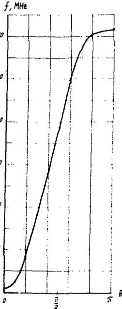
Fig. 3 Dispersion curve of a cavity loaded with washers and discs;  $\beta = 0.8$ ,  $K_c = 47\%$ .
