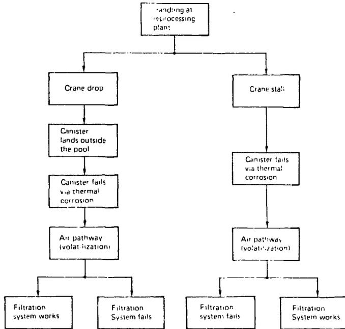
Fig. 3 EVENT TREE FOR HANDLING ACCIDENTS AT THE FUEL REPROCESSING PLANT
