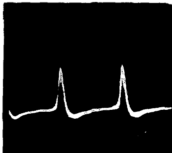
Fig. 5 Bunch signal behind the second Wideröe tank, measured with a coaxial Faraday cup (real time, 50 mV/div., 10 ns/div.).
