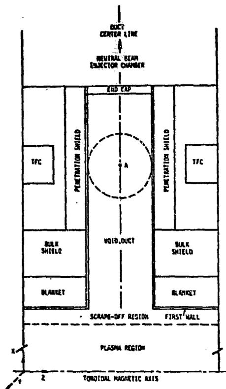
Fig. 6. Neutral beam duct model for nuclear analysis.
