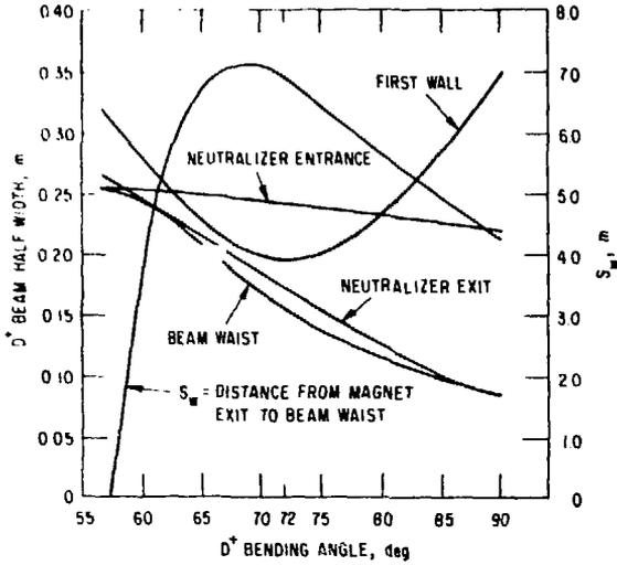
Fig. 2. Location of beam waist versus  $D^+$  bending angle, and beam half-widths at several locations. For TNS Design I.
