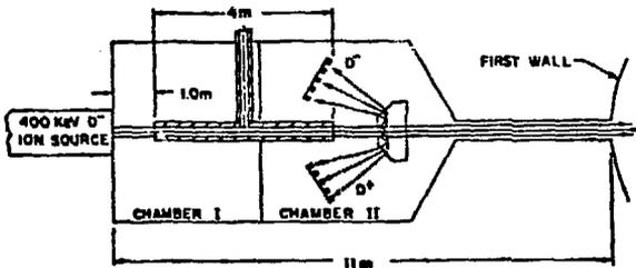
Fig. 3. Preliminary layout of a  $D^- \rightarrow D^0$  TNS beam line.
