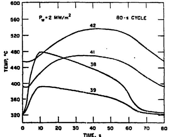
Figure 6. Temperature Response as a Function of Time for Stainless Steel First Wall with 2 MW/m² Average Neutron Wall Loading.
