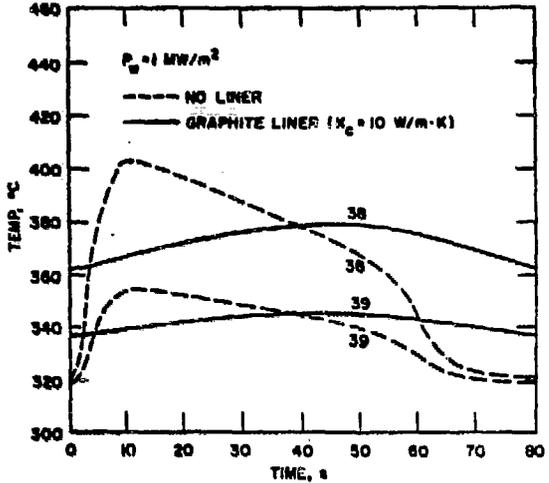
Figure 10. Temperature Response of Stainless Steel Wall With and Without Graphite Liner.
