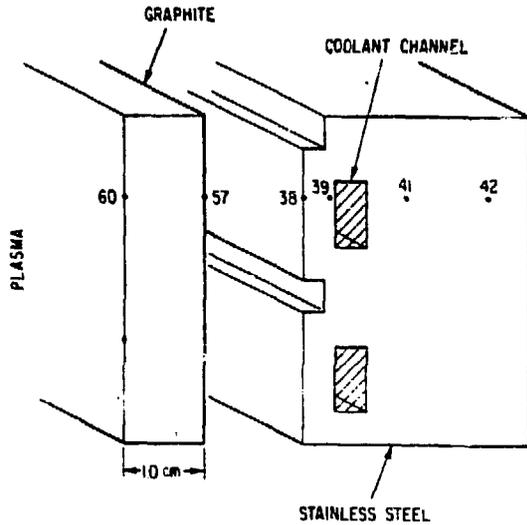
Figure 2. Schematic Diagram of First-Wall Concept With Radiatively-Cooled Graphite Liner
