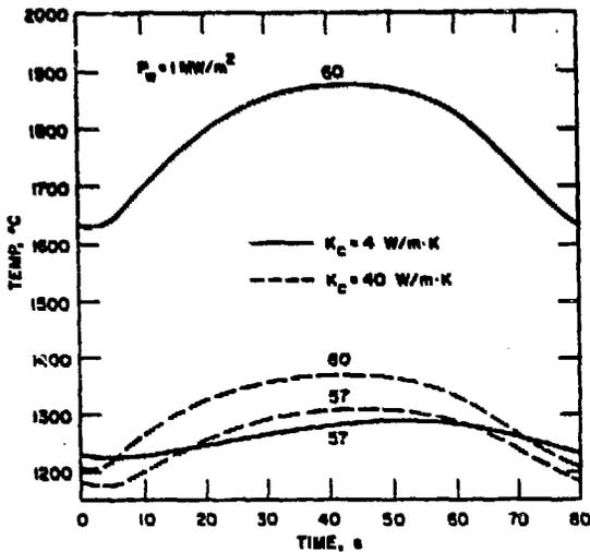
Figure 8. Temperature Response of Graphite Liner Showing Effect of Thermal Conductivity of Graphite.
