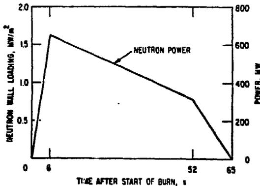
Figure 3. Power Curve for Reference Burn Cycle.
