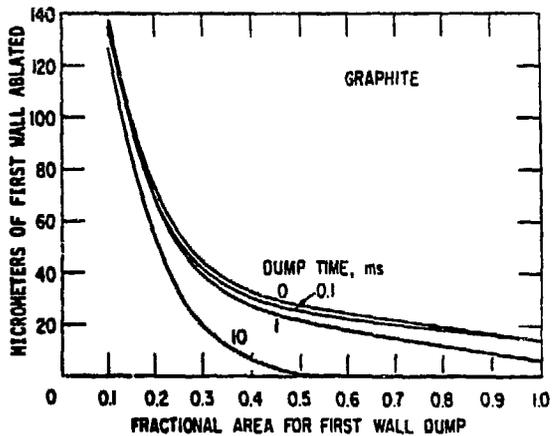
Figure 12. Thickness of Ablated Region of Graphite Wall After Plasma Disruption.
