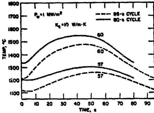
Figure 7. Temperature Response as a Function of Time for Graphite Liner During Two Burn Cycles.
