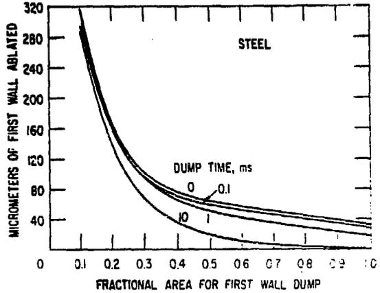
Figure 11. Thickness of Ablated Region of Stainless Steel Wall After Plasma Disruption.
